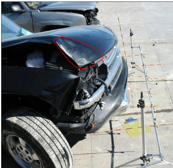
Figure 7: Case vehicle's frontal damage viewed from right along reference line; Note: damage area on front right hood possibly from contact with guardrail support post (case photo #27a)
