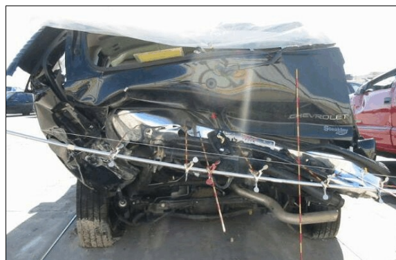
Figure 14: Non-horizontal damage to case vehicle’s back from impact with bridge pillar; Note: vehicle was airborne and upside down at time of impact and trunk was closer to the ground than the engine compartment (case photo #21a)
