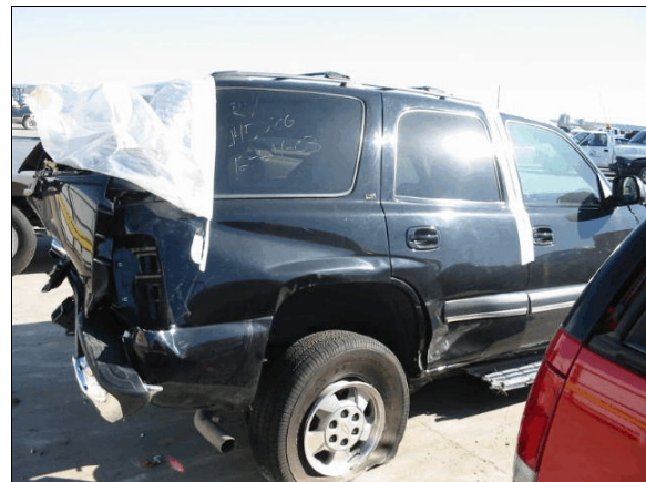
Figure 4: Damage to case vehicle's right rear door and running board most likely from sustained contact with deformed “W” beam (case photo #25)
