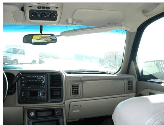
Figure 16: Case vehicle's front right seating area showing non-deployed front right air bag and no apparent evidence of occupant contact to center and right instrument panels and greenhouse area (case photo #33)
