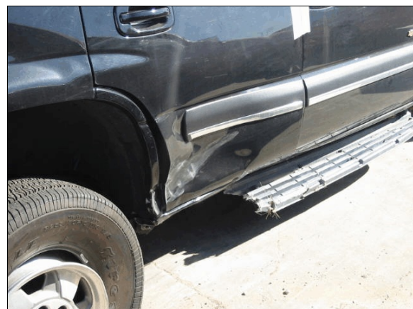
Figure 5: Close-up of damage to case vehicle's right rear door and running board most likely from sustained contact with deformed “W” beam guardrail (case photo #27)
