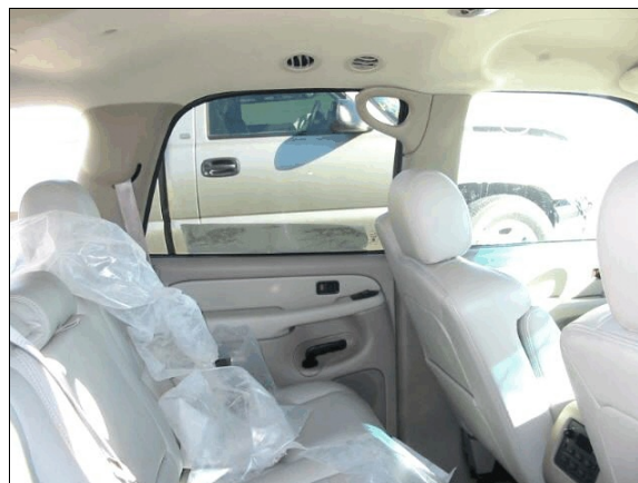
Figure 17: Case vehicle’s second seating area viewed from right showing no apparent evidence of occupant contact to roof above driver’s head and no indication of distortion or damage to driver’s seat back (case photo #34)
