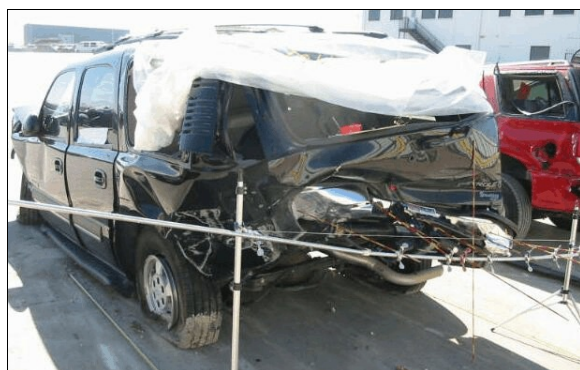
Figure 11: Non-horizontal damage to case vehicle's back from contact with bridge pillar, viewed from left of back with contour gauge set at bumper level; Note: vehicle was airborne and upside down at time of impact (case photo #19)
