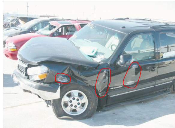
Figure 6: Case vehicle's left fender and left front door areas showing white, vertically oriented, contact evidence most likely from contact with delineator post(s) originally positioned behind guardrail; Note: left outside rearview mirror contacted front-to-back (case photo #16)
