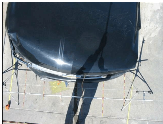
Figure 13: Overhead view of case vehicle's front damage from impact with longitudinal barrier (i.e., "W" beam guardrail); Note: crush greatest at front right corner (case photo #27d)
