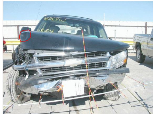
Figure 3: Case vehicle frontal damage from impact with “W” beam guardrail with contour gauge set at bumper level; Note: highlighted area on front right hood most likely from impact with guardrail support post (case photo #12)
