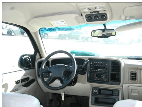
Figure 15: Case vehicle's driver seating area showing non-deployed driver air bag and no apparent evidence of occupant contact to steering wheel, instrument panel, or greenhouse areas (case photo #31)
