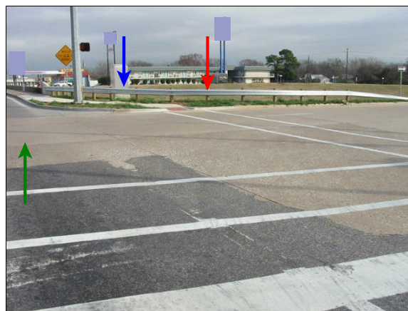
Figure 9: Arrows indicate areas of impact (green), and final rest for case vehicle (blue) and BMW (red); post-impact, case vehicle rotated counter-clockwise and BMW clockwise (case photo #09)
