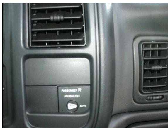
Figure 8: Case vehicle's front right passenger air bag cutoff switch showing switch located in "automatic" position; Note: with no front right passenger the seat's sensor correctly indicated that no deployment was required (case photo #33)
