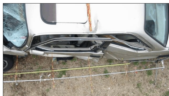
Figure 18: Overhead view of middle portion of BMW’s left side impact with contour gauge positioned above the sill (case photo #48)
