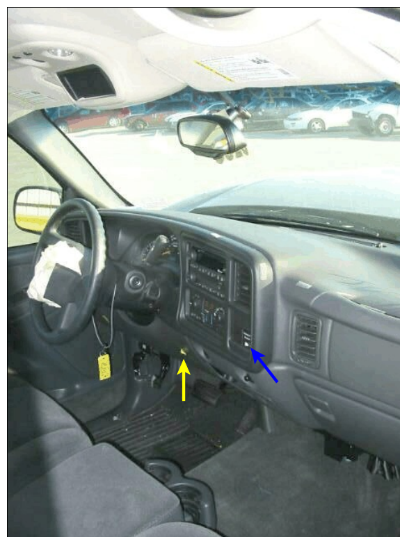
Figure 14: Vertical view of case vehicle’s front seating area showing deployed driver air bag, non-deployed front right passenger air bag, possible contact evidence on right side of driver’s knee bolster, and air bag cutoff switch (case photo #29)
