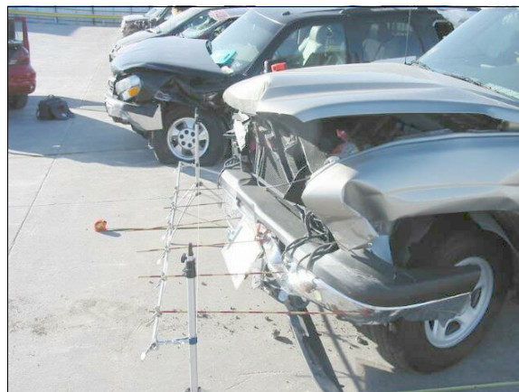
Figure 12: Case vehicle’s frontal damage viewed along reference line from left; Note: greater crush at C 1 , indicating oblique nature of case vehicle’s interaction with BMW’s left side (case photo #14)
