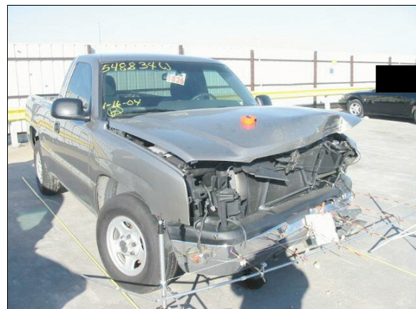
Figure 5: Case vehicle's frontal damage viewed from right of front showing direct damage extending across entire front (case photo #22)
