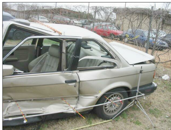
Figure 7: BMW's damaged left front door with crush extending onto left quarter panel; Note: door's window frame secured to left "B"-pillar for crush measurement purposes (case photo #46)
