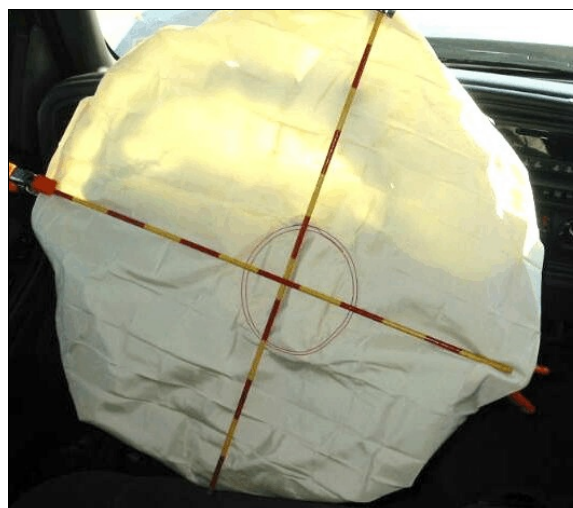
Figure 15: Case vehicle's deployed driver air bag showing no obvious evidence of occupant contact (case photo #38)
