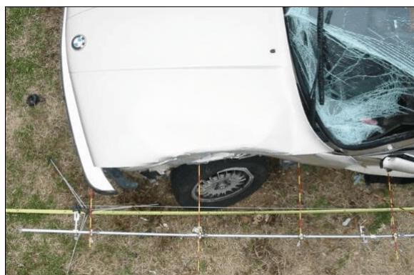
Figure 17: Overhead view of frontal portion of BMW’s left side damage with contour gauge positioned above the sill (case photo #47)
