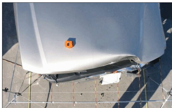
Figure 11: Overhead view of case vehicle’s frontal damage with contour gauge positioned at bumper level (case photo #23a)
