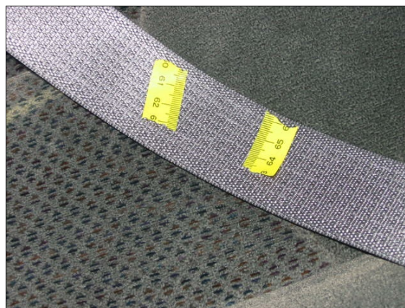
Figure 16: Loading evidence (i.e., wear mark) on webbing of case vehicle's drivers seat belt (case photo #34)
