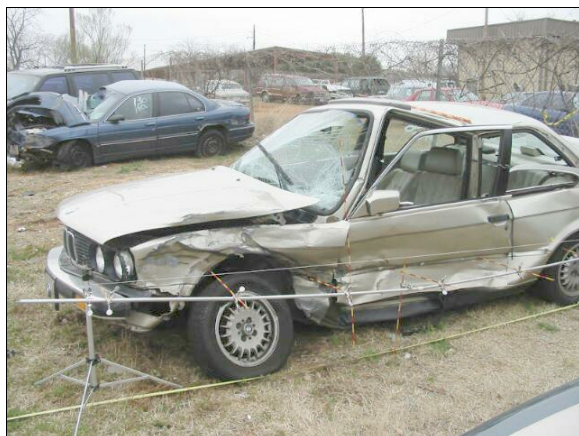
Figure 6 BMW's damaged left front half with contour gauge set above sill level; Note: damaged left front wheel assembly and direct contact to left "A"-pillar (case photo #45)
