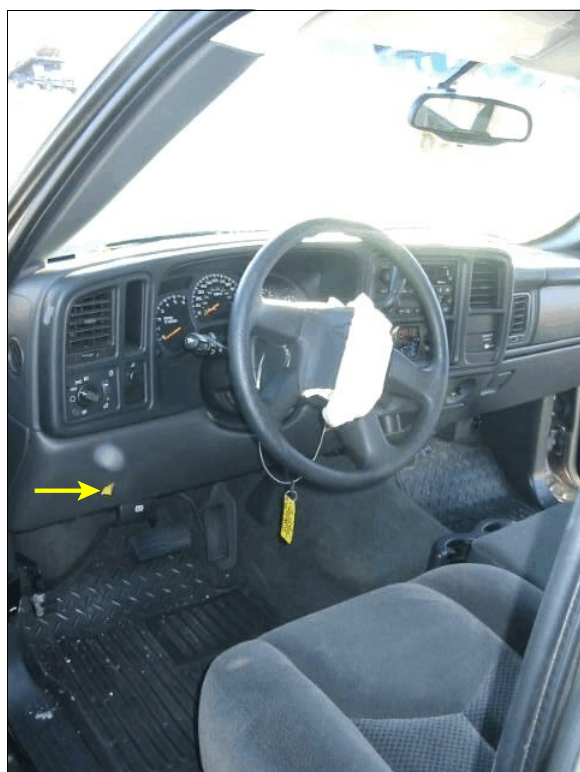
Figure 13: Vertical view of case vehicle’s driver seating area showing deployed driver air bag and only possible contact evidence on left side of driver’s knee bolster (case photo #26)
