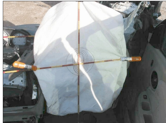
Figure 21: Front surface of case vehicle's deployed front right passenger air bag showing no obvious evidence of occupant contact (case photo #43)
