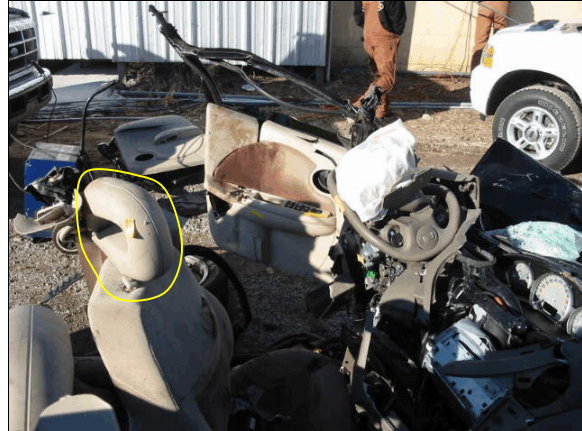
Figure 22: Elevated view of case vehicle's driver seating area showing distorted steering wheel rim, deployed driver air bag, contact evidence on interior surface of driver's door, and distortion to driver's adjustable head restraint from contact by back left passenger (case photo #28)
