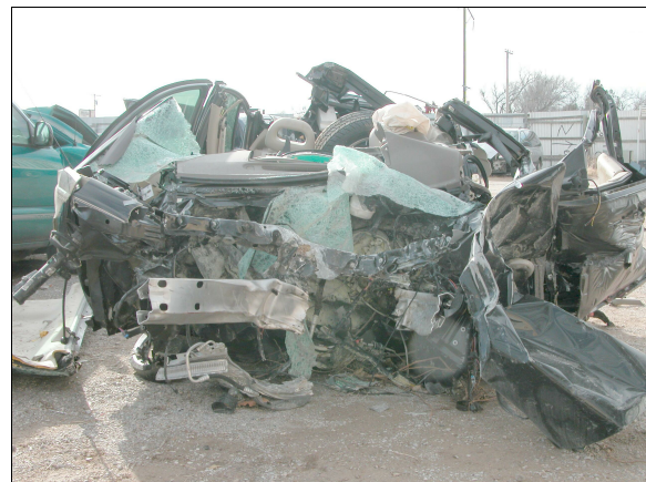
Figure 10: Frontal view of case vehicle's severely damaged front end; Note: engine was knocked out during impact with 2 nd tree (case photo #14)
