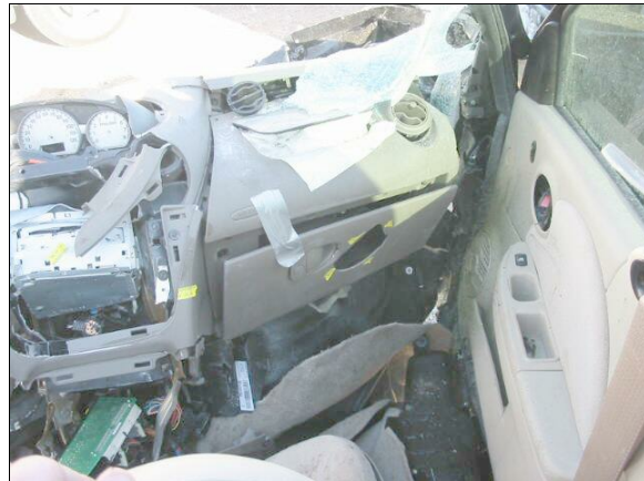
Figure 16: Case vehicle's front right passenger seating area showing deployed front right passenger air bag, intrusions, and contact evidence; Note: contacts to center instrument panel and "hole" in glove box door (case photo #24)
