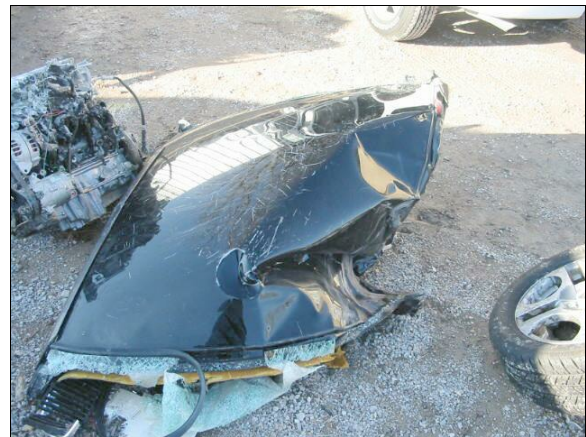
Figure 9: Damage to case vehicle's roof, removed by rescue personnel, showing indentation over driver's seating area from contact with horizontal portion of fence pole; Note: separated engine block in background (case photo #16)
