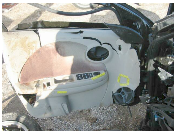
Figure 14: Interior surface of case vehicle's driver front door showing evidence of occupant contact (case photo #25)
