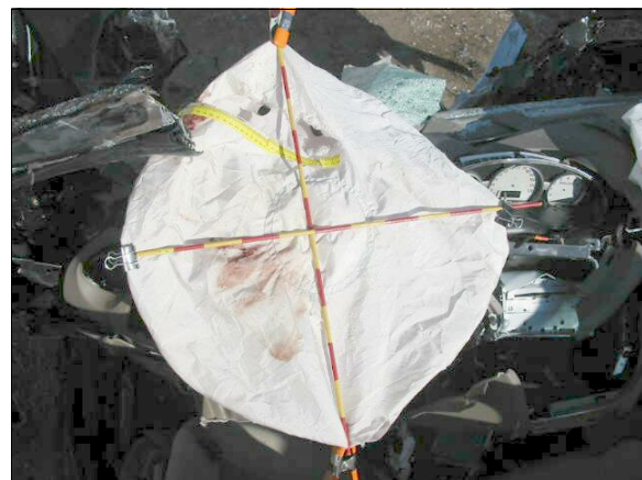
Figure 19: Front surface of case vehicle's deployed driver air bag showing contact evidence near center in lower left quadrant and tear in air bag's fabric in upper left quadrant (case photo #30)
