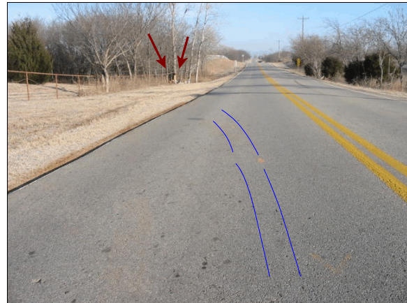
Figure 3: Curved marks (highlighted) from case vehicle's right side tires as vehicle travels northward in southbound lane heading off road onto west roadside and impact area (arrows) with fence rail and trees (case photo #03b)
