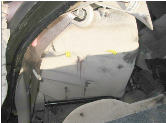
Figure 17: Back surface of case vehicle's driver seat back showing contact evidence from impact by back left occupant (case photo #27)
