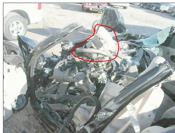
Figure 13: Case vehicle's driver seating area viewed from behind left "B"-pillar showing intrusions and contact evidence; Note: deformed steering wheel and deployed driver air bag (case photo #20)
