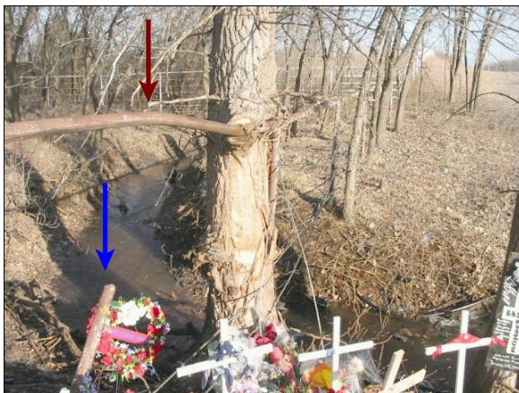
Figure 8: Close-up of 2 nd tree impacted (4 th event) by case vehicle; arrows show impact with fence post, blue arrow—3 rd event, and fence rail, red arrow—5 th event (case photo #09)
