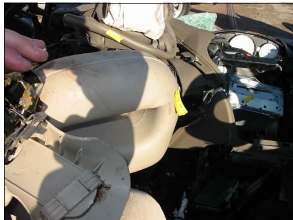
Figure 18: Close-up of back surface of adjustable head restraint for case vehicle's driver showing distortion and damage caused by contact from back left occupant; Note: distorted steering wheel rim in background (case photo #48)
