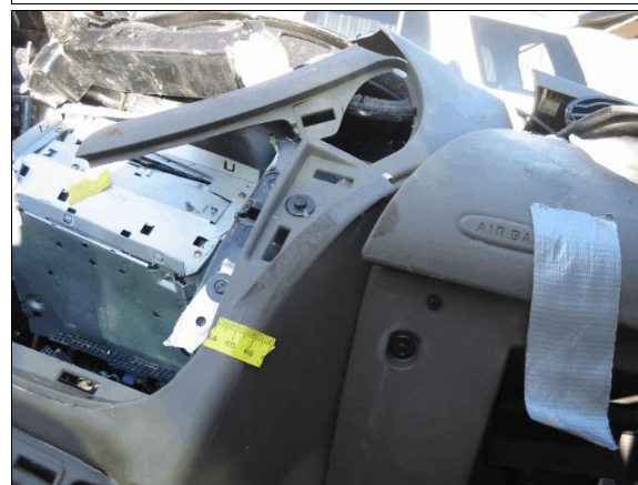
Figure 15: Contact evidence on case vehicle's center instrument panel area; Note: deployed front right passenger air bag (case photo #23)
