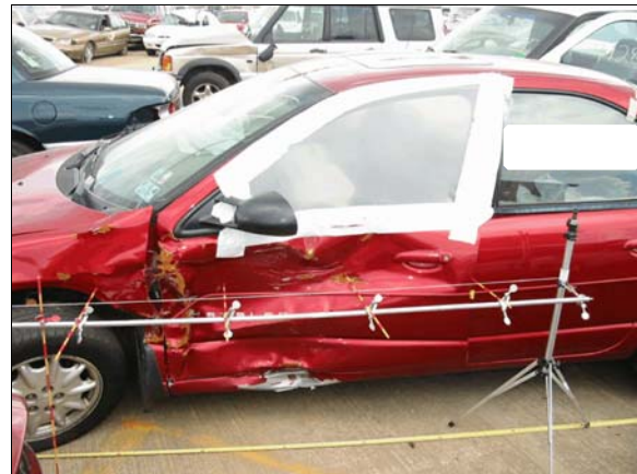
Figure 15: Chrysler's damaged left fender and left front door from impact with case vehicle
