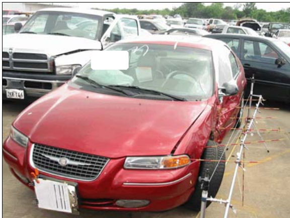
Figure 14: Left front corner view of damage to left side of Chrysler from impact with case vehicle
