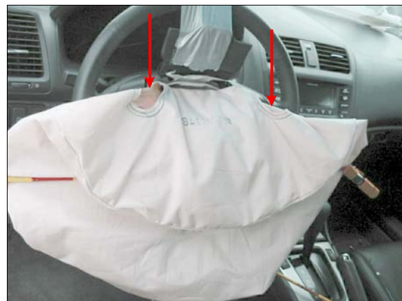
Figure 12: Case vehicle driver's air bag vent ports
