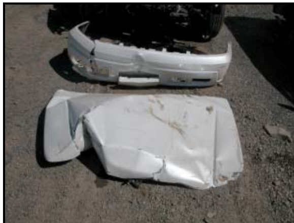
Figure 6: Damaged bumper fascia and reinforcement.
