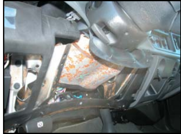
Figure 7: Deformation of the metal backer behind the knee bolster.
