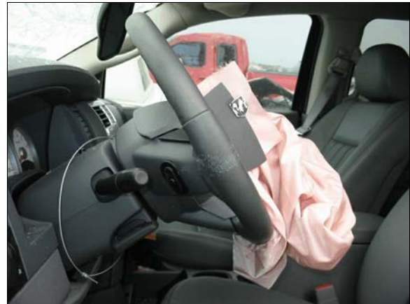
Figure 12: Overview of case vehicle's steering wheel and steering column; Note, spots on steering wheel rim are from adhesive tape
