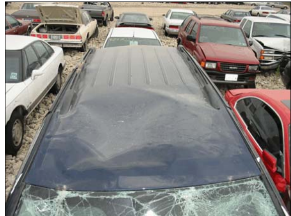
Figure 5: Rollover damage to the top
