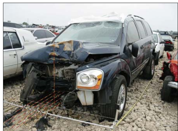
Figure 7: Overview of front and left side of case vehicle and damage to front of vehicle from impact with the utility pole
