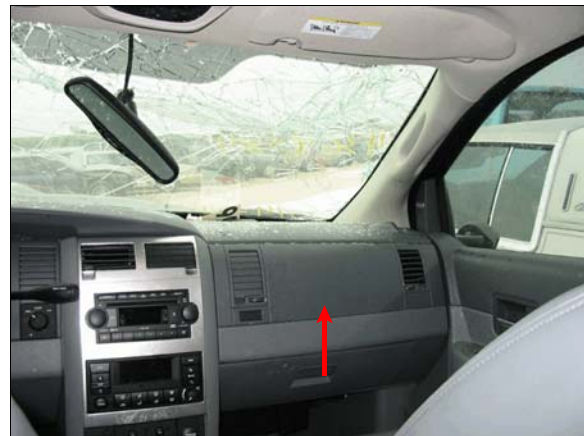
Figure 16: Overview of case vehicle's right instrument panel and location of front right air bag (arrow)
