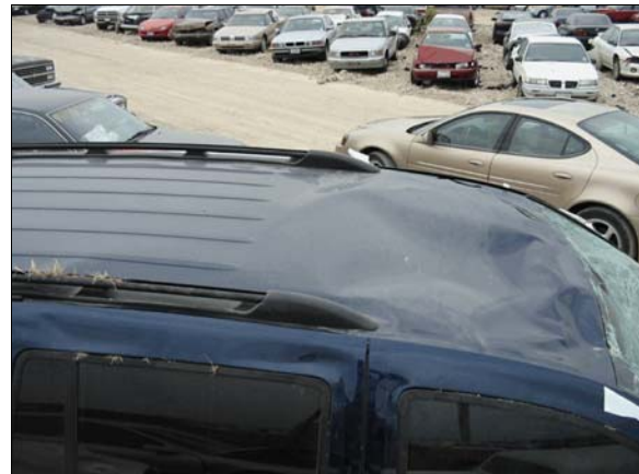
Figure 10: Rollover damage to right roof side rail and roof
