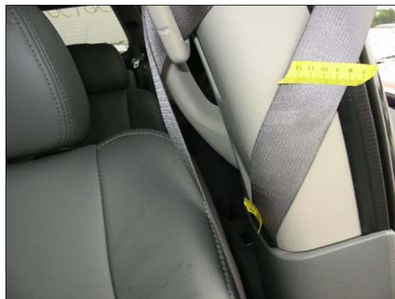
Figure 18: Load marks on driver's shoulder belt, between the yellow tapes
