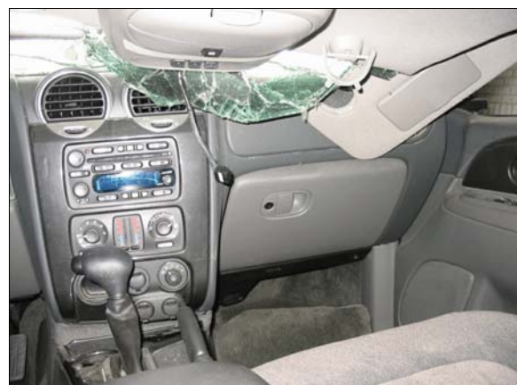
Figure 10: Center and right instrument panel; front right air bag module cover just above glove box door
