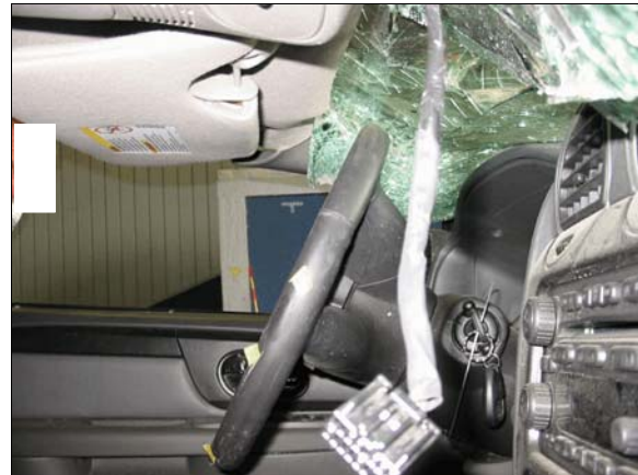
Figure 8: Right side view of steering wheel and steering column showing no deformation
