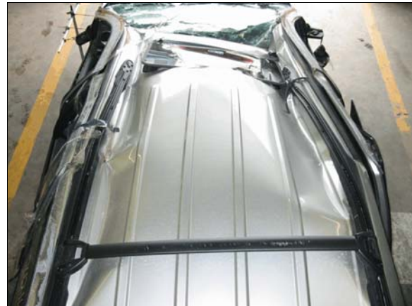
Figure 6: Crush to the case vehicle's roof from rollover; view from back of vehicle
