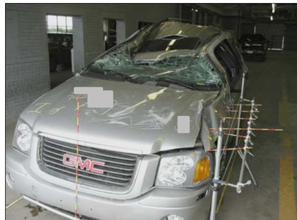
Figure 7: Roof crush, hood scratches and pavement grinding to A-pillars and roof rails from rollover
