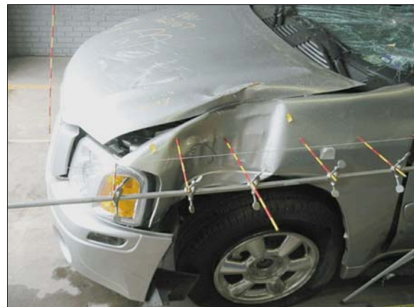
Figure 5: Damage to case vehicle's left fender and left front wheel from impact with luminaire pole
