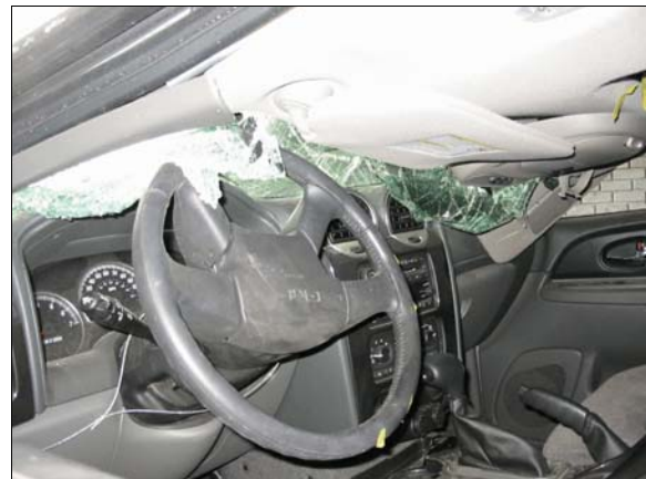
Figure 9: Intrusion into driver’s occupant space and overview of steering wheel ( rotated 180 degrees) and instrument panel
