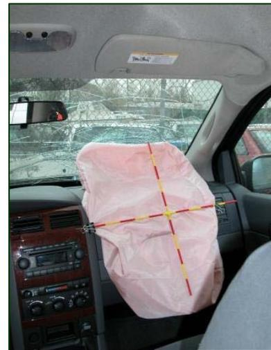
**Figure 12. Front right passenger’s trajectory and deployed air bag.**
