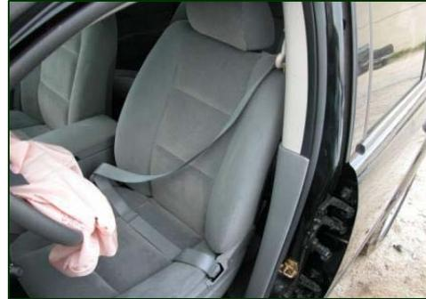
**Figure 9. Locked position of the driver's safety belt webbing.**
