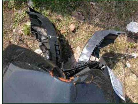
**Figure 5. Overhead view documenting the extent of frontal crush.**
