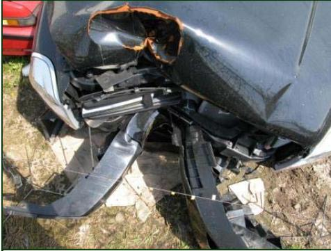
**Figure 4. Frontal damage to the Dodge Durango.**
