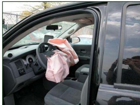
**Figure 6. Deployed CAC Frontal air bags.**
