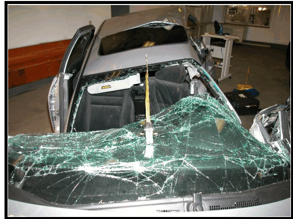
Figure 6. Overview of vehicle intrusion
