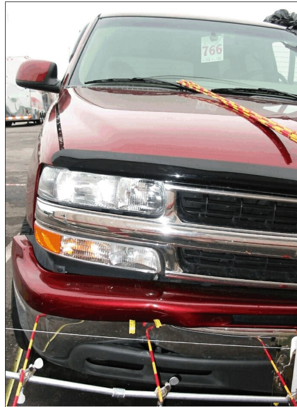
Figure 13: Case vehicle's impact (5 th event) with corner of concrete bus bench (case photo #20)
