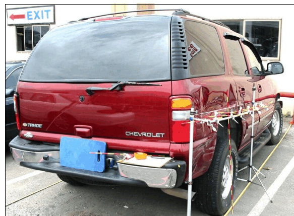
Figure 20: Case vehicle's right quarter panel damage (6 th event) most likely from impact with bus stop sign post viewed from right of back (case photo #38)
