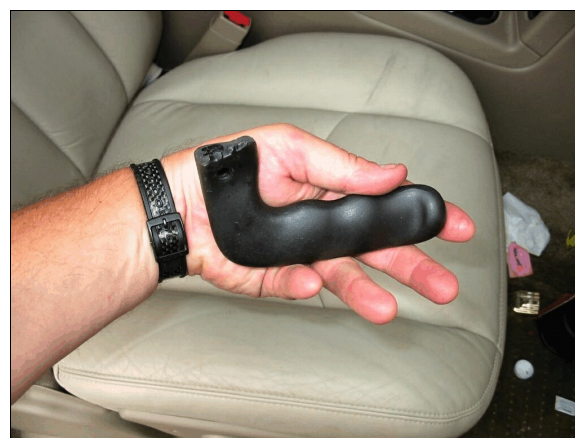
Figure 24: Broken off door handle from case vehicle's driver door (case photo #57)
