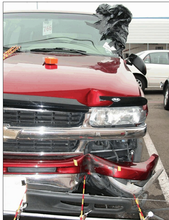
Figure 12: Case vehicle’s impact (4 th event) with protective corner post (case photo #22)
