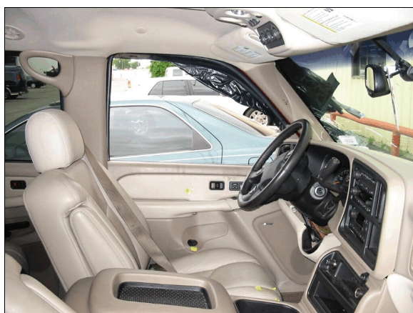
Figure 21: Case vehicle's driver seating area viewed from right showing contact evidence on driver's door (yellow tape) and blood on driver's seat (case photo #51)
