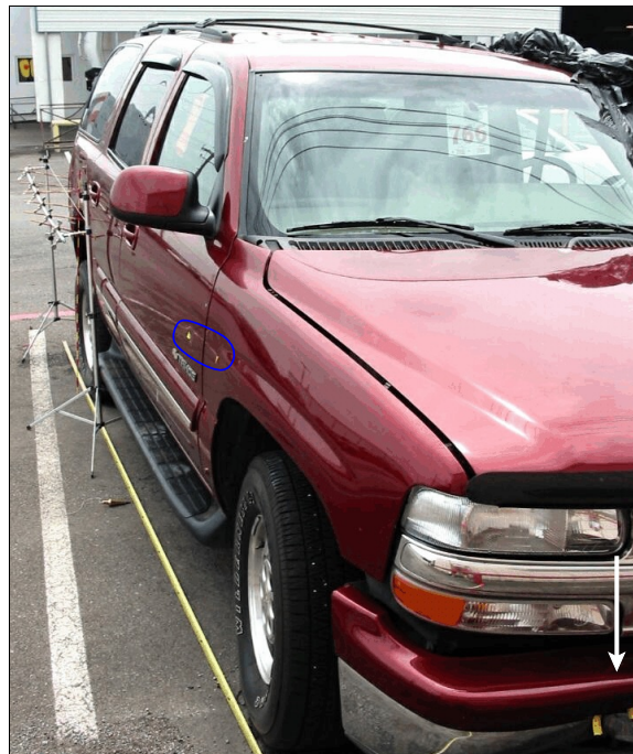
Figure 16: Case vehicle's impact with corner of concrete bus bench (arrow), unknown damage—current versus prior, near right "A"-pillar, and damage to right quarter panel from bus stop sign post (case photo #44)
