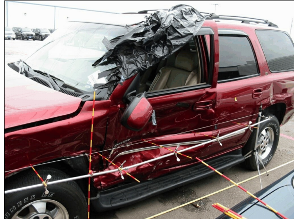
Figure 7: Case vehicle's initial (1 st event) left side damage showing C 1 through C 3 crush positions with contour gauge positioned above sill level (case photo #29)
