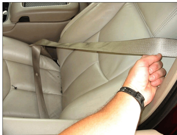
Figure 29: Case vehicle's driver seat belt webbing showing loading evidence-waffling (case photo #61)
