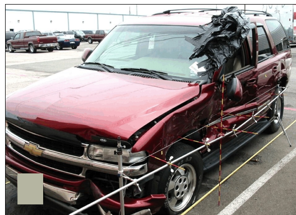
Figure 6: Case vehicle's initial (1 st event) left side damage from impact by front of Chrysler (case photo #27)
