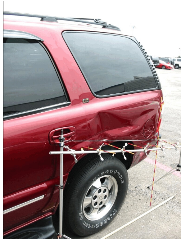
Figure 10: Case vehicle’s left side slap damage (2 nd event) from impact with Chrysler’s right side (case photo #33)
