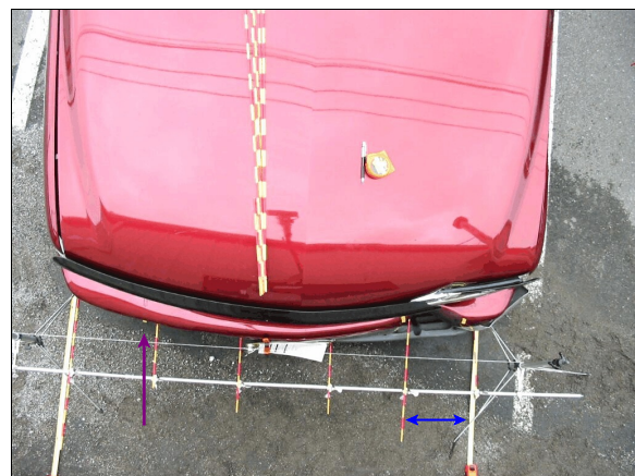
Figure 19: Overhead view of case vehicle's frontal impacts (i.e., post-blue arrows, bench-grape arrow) with contour gauge positioned at bumper level (case photo #23)
