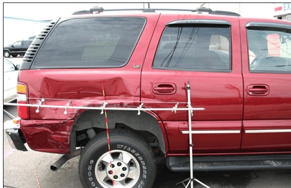
Figure 15: Case vehicle's right quarter panel damage (6 th event) most likely from impact with bus stop sign post with contour gauge positioned above sill (case photo #40)
