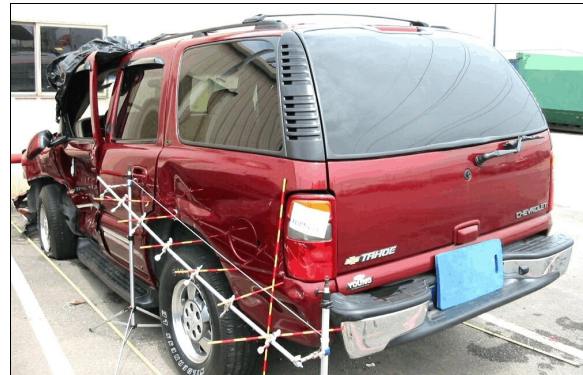
Figure 18: Case vehicle's left side slap damage (2 nd event) viewed from left of back (case photo #36)
