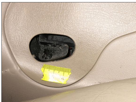
Figure 23: Close-up of area where case vehicle's driver door handle was broken off driver's door (case photo #55)
