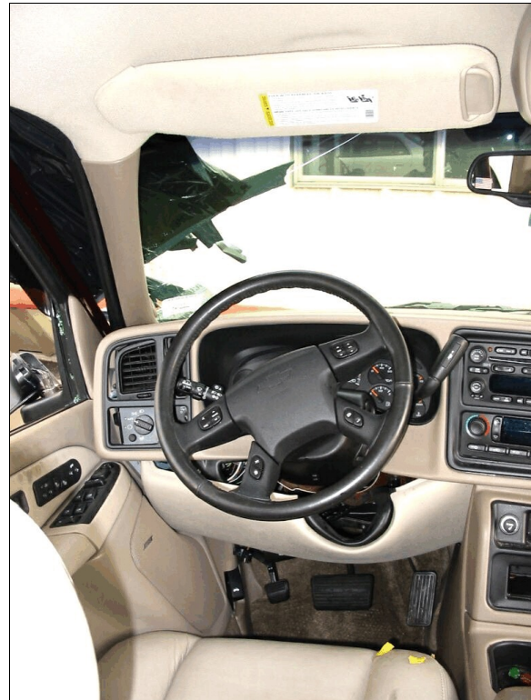
Figure 27: Vertical view of case vehicle's driver seating area showing non-deployed driver air bag, intrusion to lower instrument panel, and blood on front right edge of driver's seat (case photo #48)
