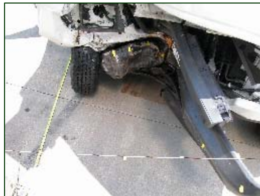
Figure 7. Maximum crush located inboard of the right corner.
