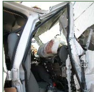
Figure 9. Lateral view of the intrusion into the front right occupant's space.
