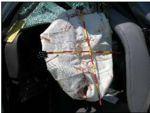
Figure 10. Deployed driver’s air bag.
