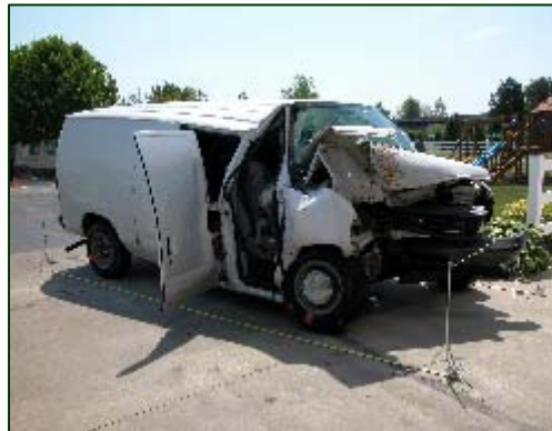
Figure 1. Front right view of the tree impact damage to the Ford E-250 cargo
