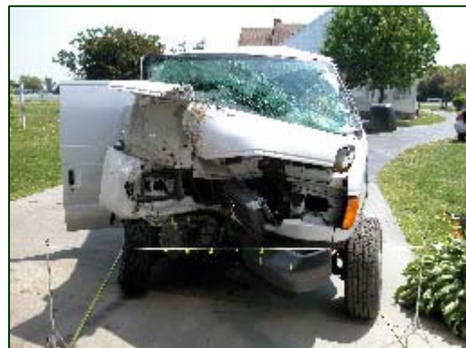
Figure 5. Frontal damage from the overlapping impacts.
