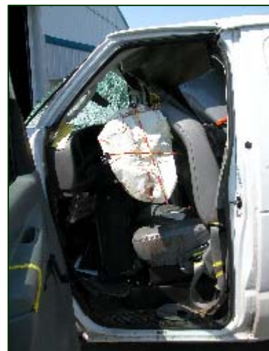
Figure 8. Lateral view of the driver's contact points and interior deformation.
