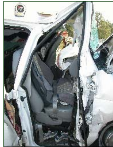
Figure 15. Position of the child passenger with respect to the deployed air bag and frontal intrusion.
