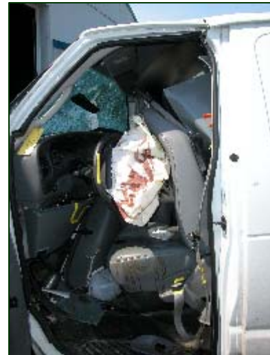
Figure 14. Driver loading of the belt system and steering wheel rim.
