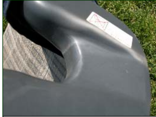
Figure 13. Belt abrasion to the right belt path of the CSS.
