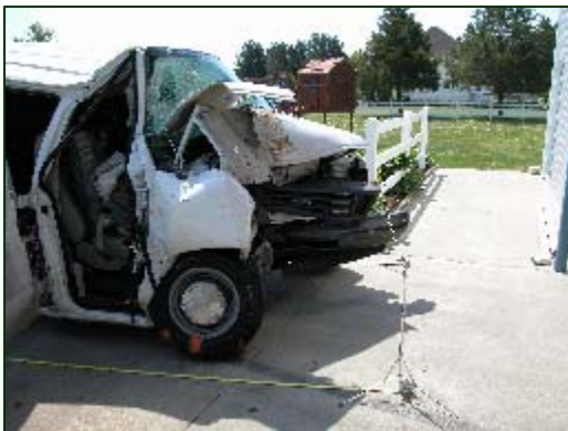
Figure 6. Lateral view documenting the extent of frontal crush.
