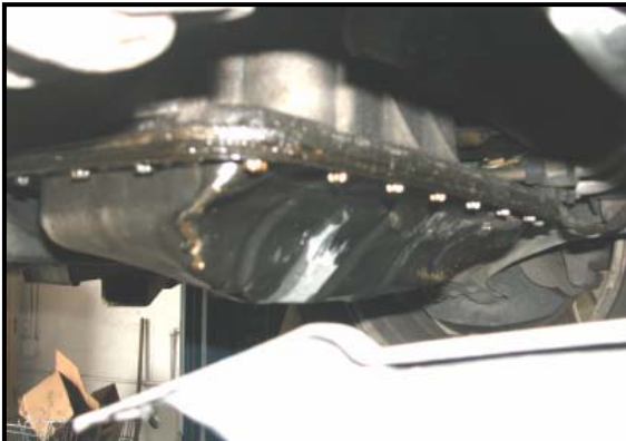
Figure 9: Right view of the deformed oil pan.
