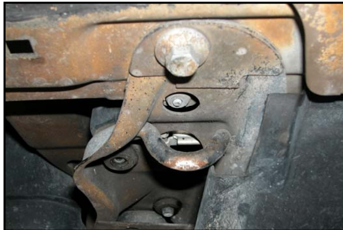
Figure 7: Close-up of the right tow hook.
