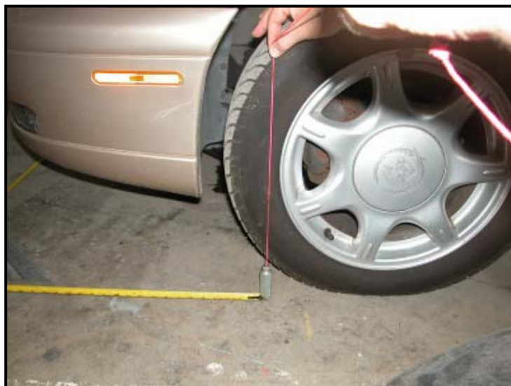
Figure 11: Depiction of the location of the oil pan's forward bolt line.
