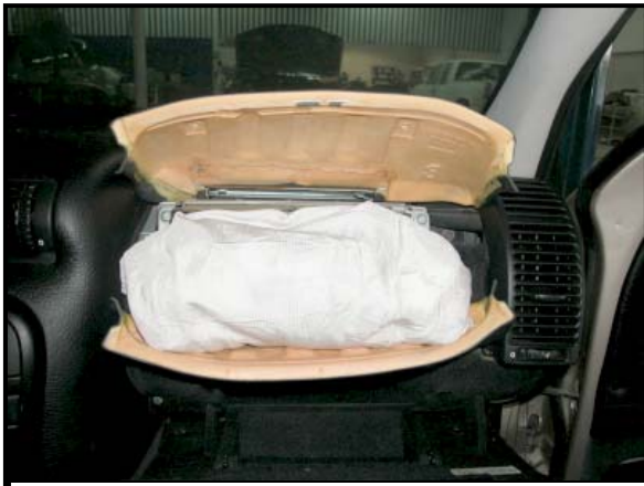
Figure 14: View of the deployed front right air bag cover flap.
