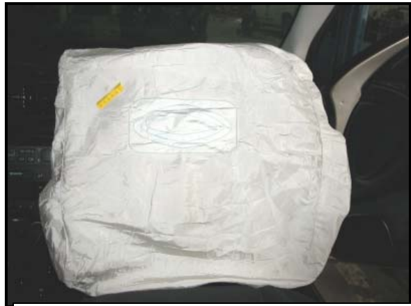
Figure 15: View of the deployed PAB.
