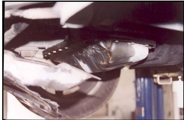
Figure 10: Left view of the deformed oil pan.
