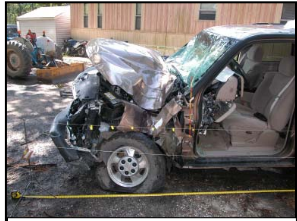
Figure 7: Residual crush at the left front fender.
