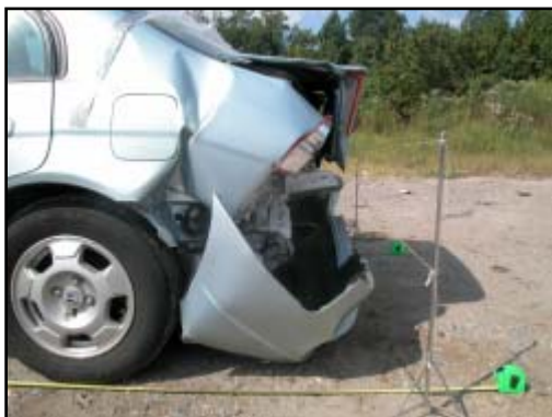
Figure 4. Lateral view of the crush and damaged left rear quarter panel
