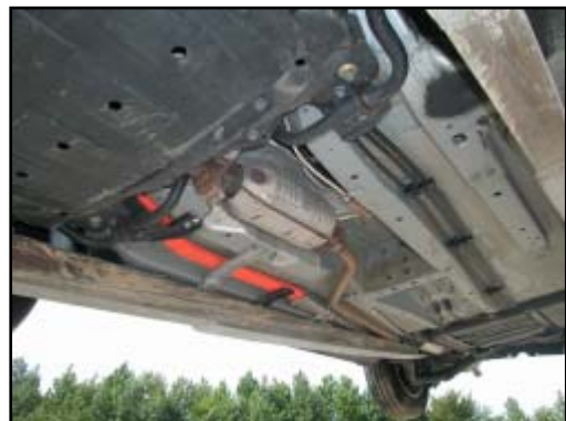
Figure 13. View of undercarriage from front left showing orange electric cables (right side)
