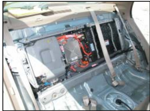
Figure 12. View of IPU compartment (rear seat and IPU cover removed)
