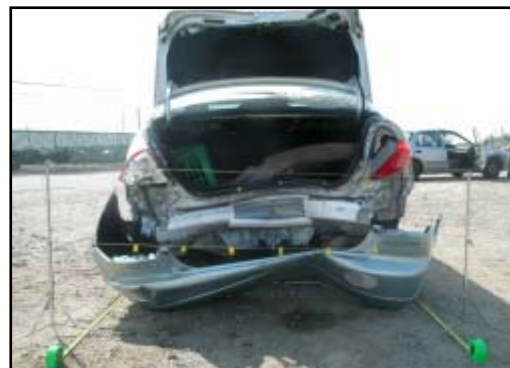
Figure 5. View of crush profile along bumper beam and trunk lip
