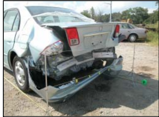
Figure 3. Rear damage to the 2003 hybrid Civic
