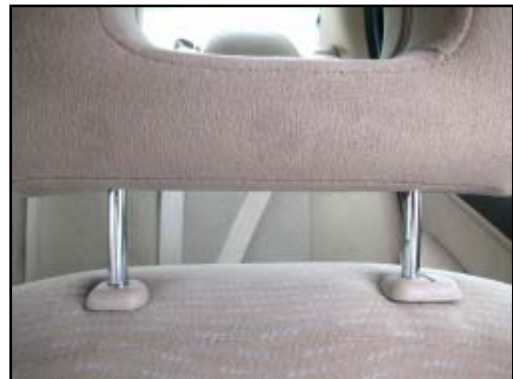
Figure 4. Close-up of driver's head restraint and displaced plastic covers
