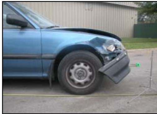
Figure 9. View of previous damage to the right front fender
