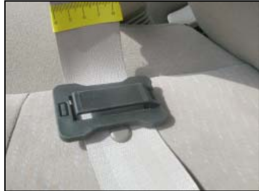
Figure 11. Close-up of after-market safety belt adjuster
