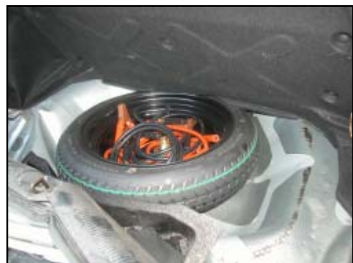
Figure 7. View from rear right corner showing the post-crash position of the spare tire
