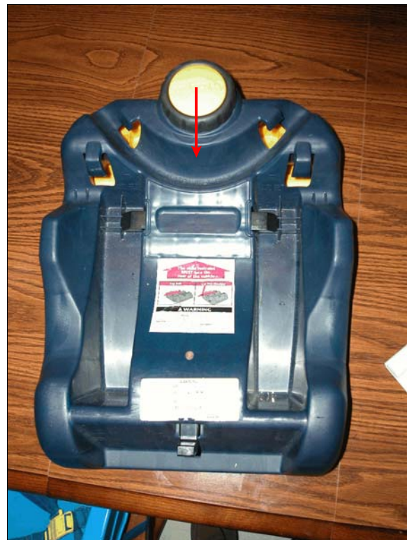
Figure 21: The infant seat base, an Evenflo model number 639004P1, arrow shows route for separate “LATCH belt”
