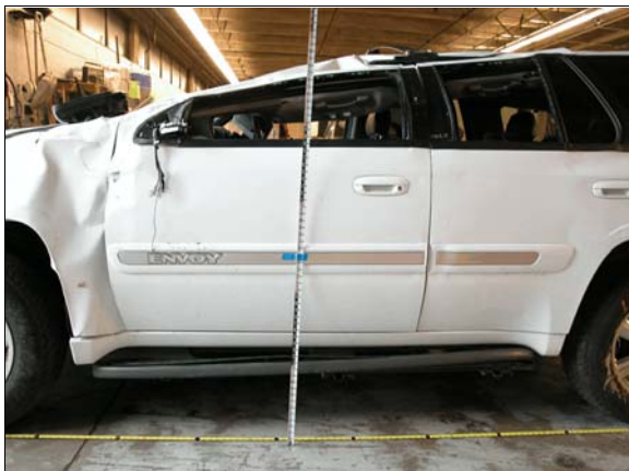
Figure 8: Crush to case vehicle’s left front roof, each black mark on yellow tape and black/white section on vertical scale=0.31 meter (1 ft)
