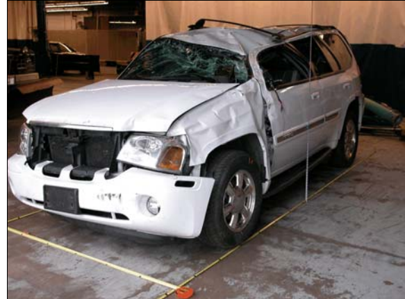
Figure 7: Overview of rollover damage to case vehicle’s front, top and left side
