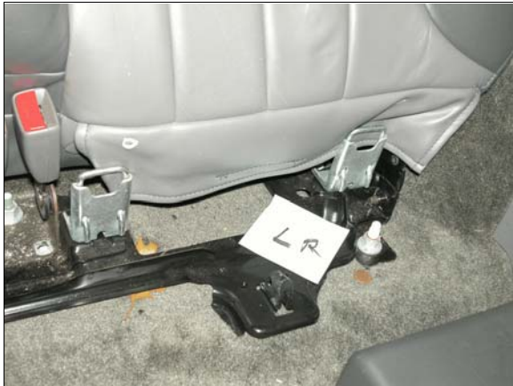
Figure 16: Lower anchors of case vehicle’s LATCH system at back left seat position, seat cushion has been folded forward
