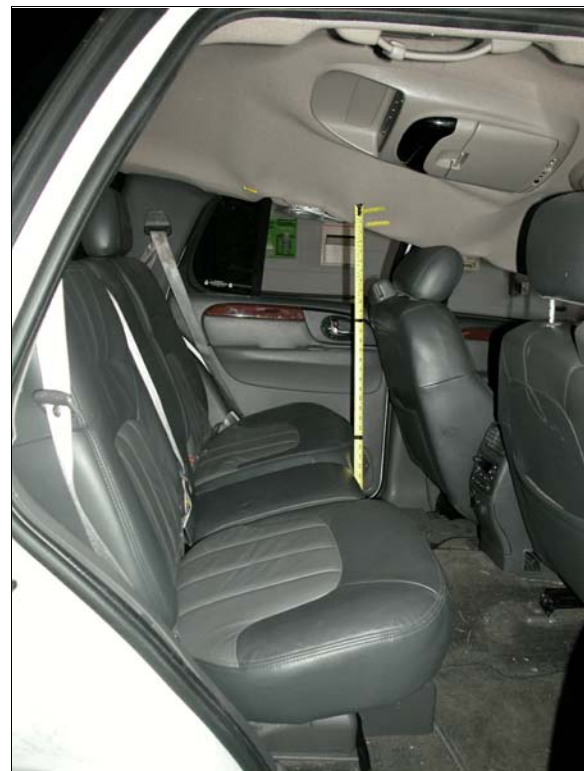
Figure 11: Overview of back seat and roof intrusion to back left seat position
