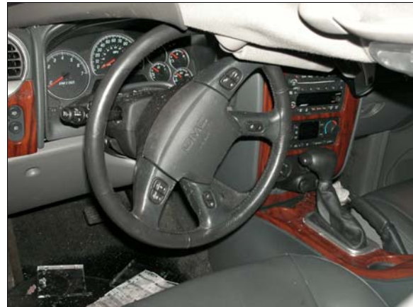
Figure 12: Overview of case vehicle's steering wheel and steering column, and intrusion of left A-pillar, roof side rail and roof
