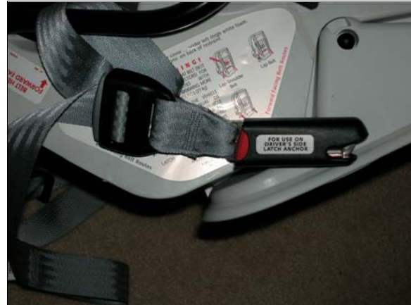
Figure 17: Child seat’s right LATCH anchor buckle and strap
