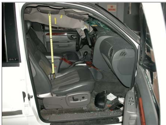
Figure 10: Overview of front right seating area and roof intrusion into driver’s seating area, each black mark on tape measure = .31 meter (1 ft)
