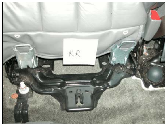
Figure 22: Lower anchors of case vehicle’s LATCH system at the back right seat position, seat cushion has been folded forward
