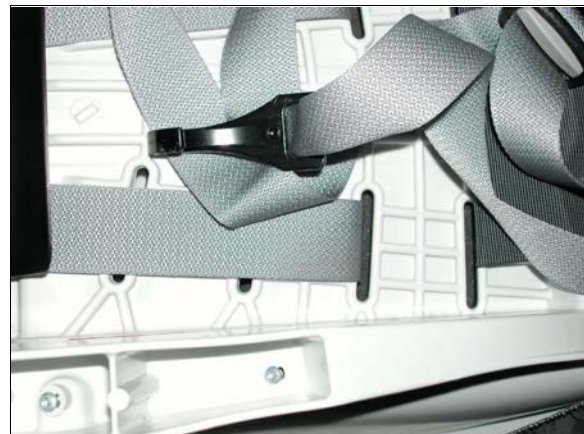
Figure 19: Close view of back left child safety seat’s tether clip and strap
