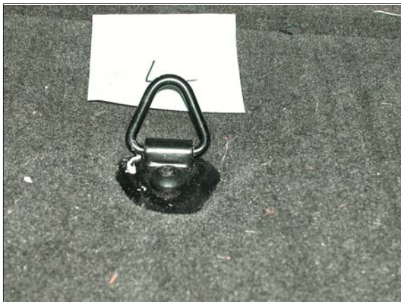
Figure 18: Case vehicle’s back left tether anchor, its located in cargo area behind back left seat
