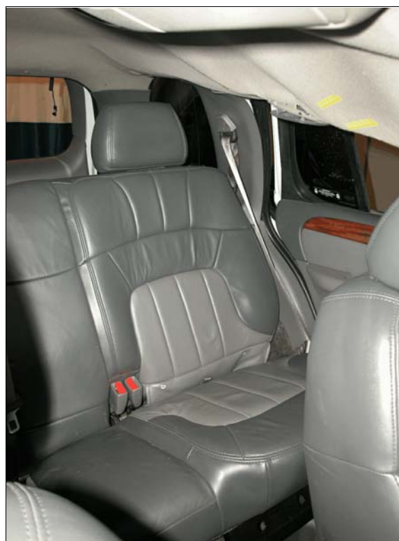
Figure 23: Overview of back left seat position, child safety seat was secured in this position by the case vehicle’s LATCH system
