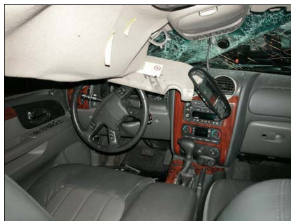
Figure 25: Overview of driver’s seating area and roof intrusion, yellow tape shows area of driver’s head contact
