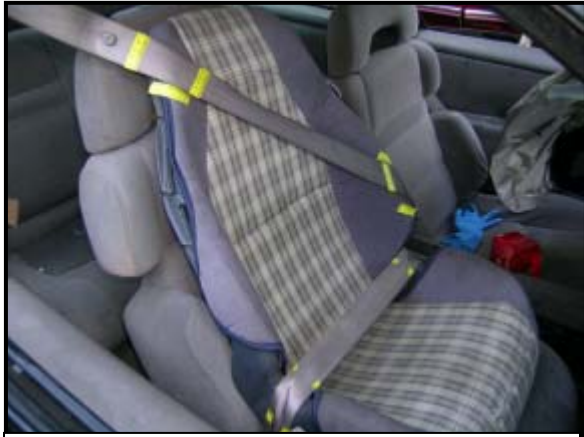
Figure 14: View of the reconstructed position of the safety belt.
