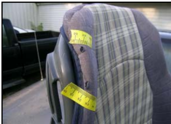
Figure 12: Close-up view of the fabric and shell abrasions caused by the locked shoulder belt.
