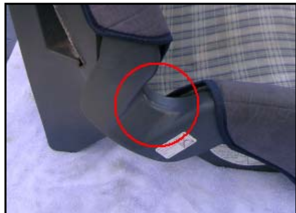
Figure 13: Close-up view of the left side shell abrasion caused by the locked lap belt.
