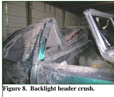
The driver's door was jammed closed by the exterior deformation. Rescue personnel opened the left front door to remove the driver's body from the vehicle. The left rear and right side doors were jammed in the closed positions. The tailgate remained intact and operational post-crash.
