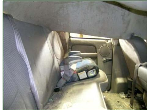
**Figure 13. Lateral view across the rear seat area and the roof intrusion.**
