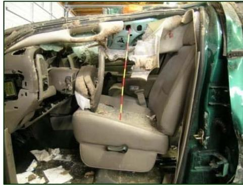
**Figure 11. Intrusion of the driver's compartment.**
