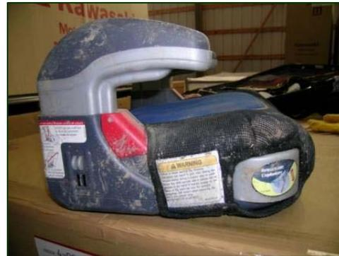
Figure 10. Right side belt path of the booster seat.
