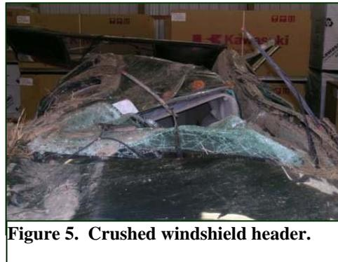
**Figure 5. Crushed windshield header.**
