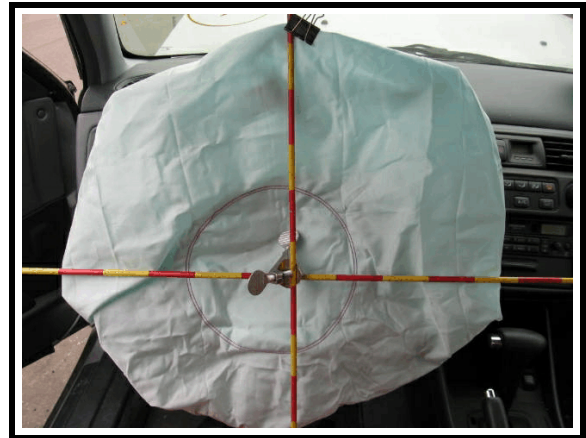
Figure 8. Deployed driver's air bag
