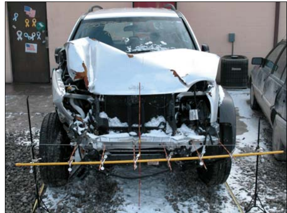
Figure 3: Damage to the front of Jeep due to impact with the left side of the case vehicle
