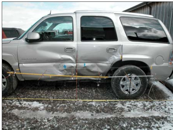
Figure 4: Damage to case vehicle's left side, each black mark on tape is 0.31 meter (1 foot), each increment on rod is 5 cm (2 in)
