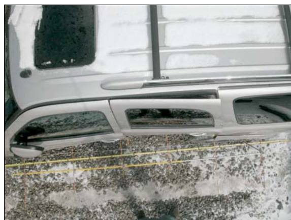
Figure 7: Top view of crush to left side of case vehicle
