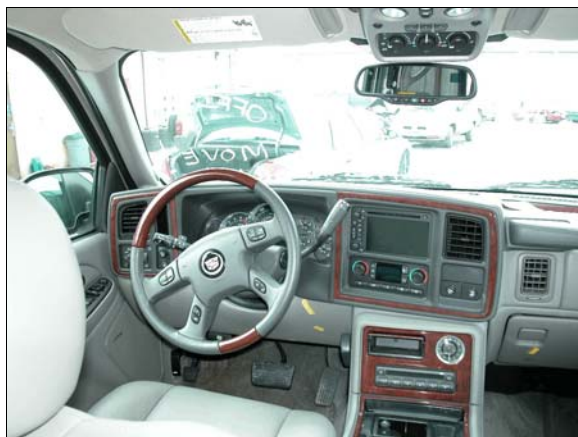
Figure 8: Overview of steering wheel, windshield and instrument panel, yellow tape shows possible occupant contact scuffs on driver’s knee bolster
