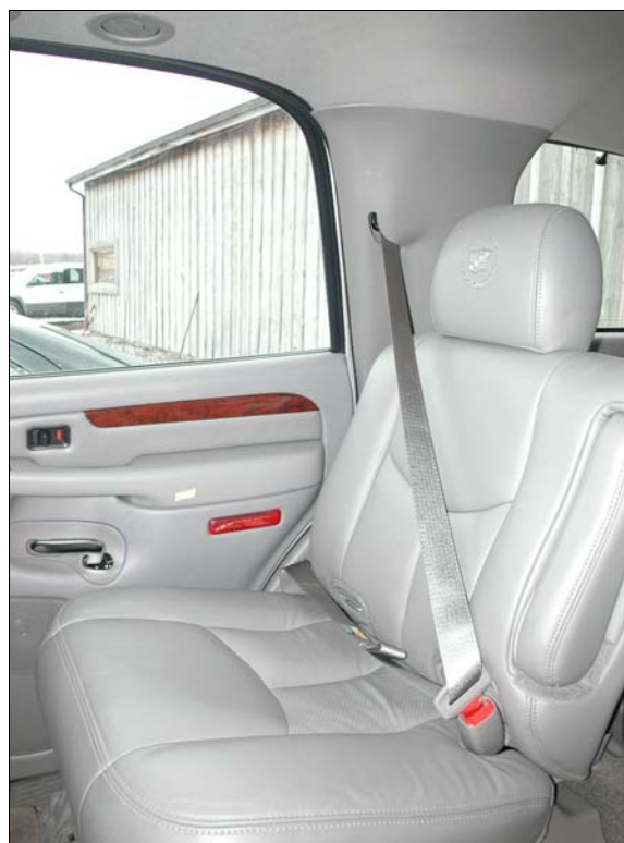
Figure 16: Overview of case vehicle's second row, right seat with safety belt buckled
