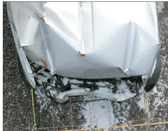
Figure 18: Top view of crush to front of Jeep
