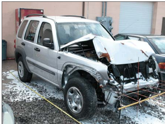
Figure 17: Right front view of damage to front of Jeep due to impact with the case vehicle
