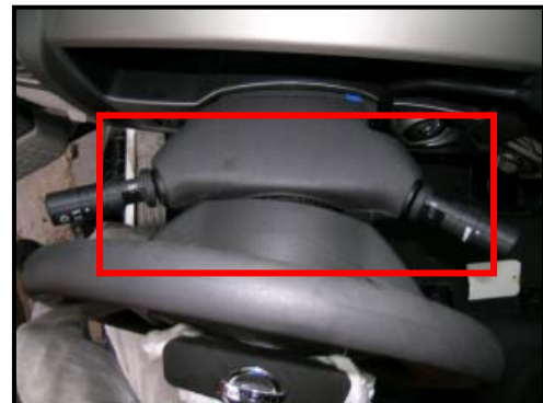
Figure 5: Overhead view depicting the deformed steering wheel mounting flange.
