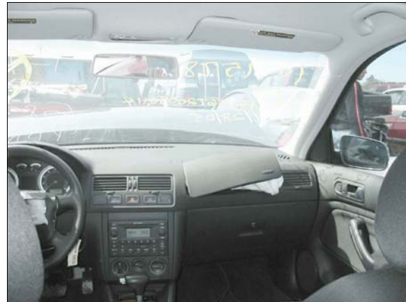
Figure 10: Overview of case vehicle's front right instrument panel and location of front right passenger air bag
