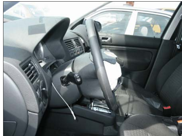
Figure 6: Left side view of case vehicle’s steering assembly showing lack of deformation
