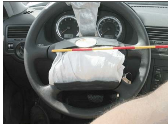
Figure 8: Case vehicle's driver air bag module flaps
