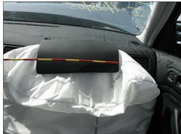
Figure 12: Case vehicle's front right passenger air bag cover flap
