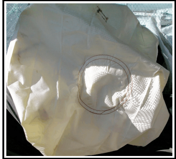
Figure 9. Deployed driver's air bag
