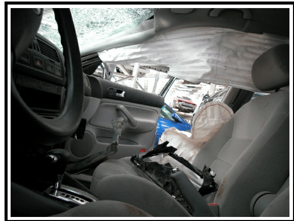
Figure 6. Front right occupant's side air curtain and side air bag
