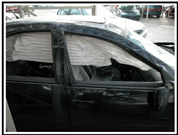
Figure 5. Exterior view, right side air curtain for front and rear seats
