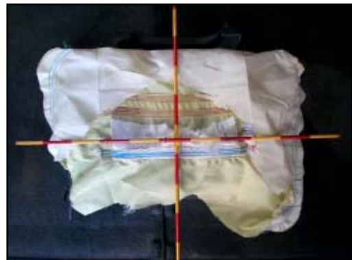
Figure 11. Driver's knee air bag (cut from module). Rear aspect of knee bolster is below air bag.
