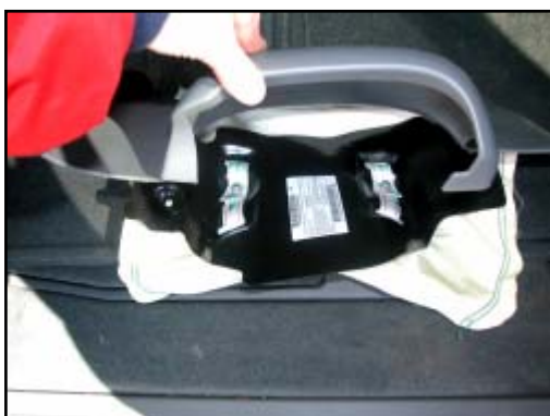
Figure 12. Top of knee bolster/air bag looking down, showing metal plate and attachment straps
