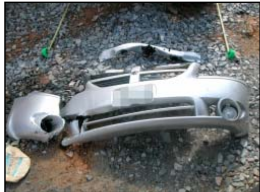
Figure 7. Front aspect of fascia, grille, and separated upper radiator support
