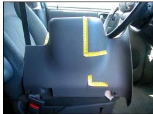
Figure 9. Close-up of damaged knee bolster
