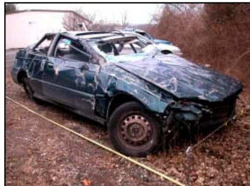
Figure 7. Right side rollover damage
