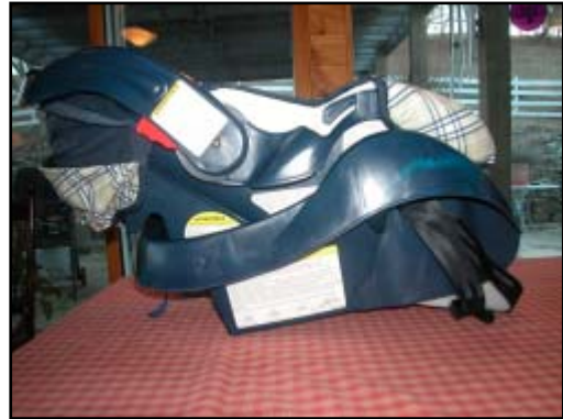
Figure 12. Left side (with respect to installation in vehicle) showing stress mark in base
