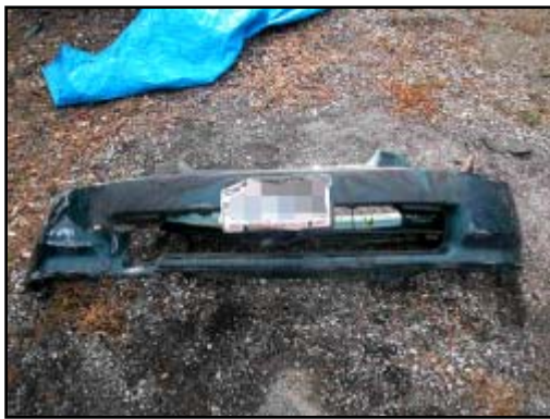
Figure 4. Separated front bumper fascia
