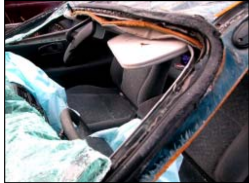
Figure 8. Windshield damage from left side
