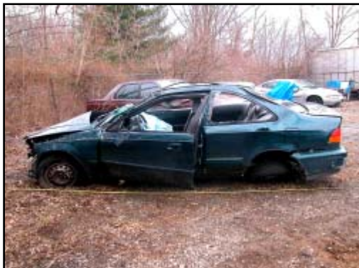
Figure 6. Left side rollover damage
