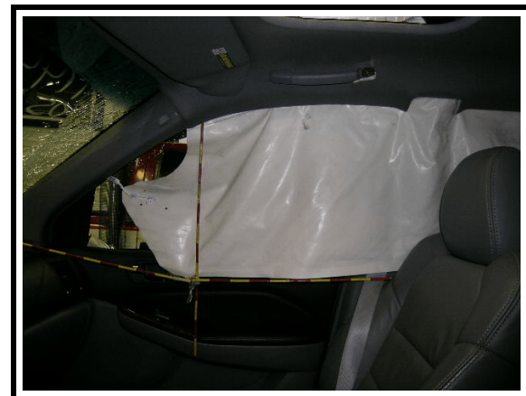
Figure 16. Right front section of the deployed right side curtain
