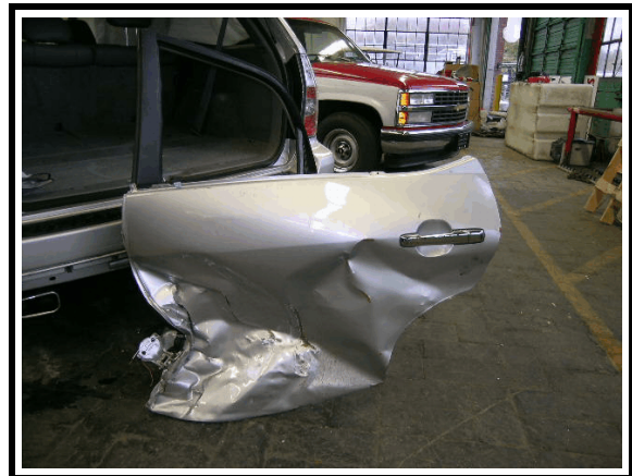
Figure 8. Left rear door damage - 2005 Acura MDX
