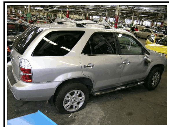
Figure 2. Right side rollover damage - 2005 Acura MDX
