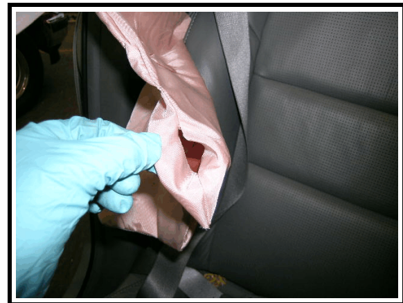
Figure 18. Side air bag vent port type
