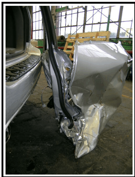
Figure 11. Left rear door, lower hinge still attached
