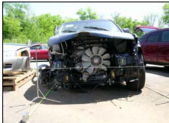
Figure 6. Frontal damage from the second utility pole impact.
