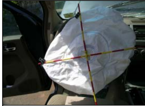
Figure 8. Deployed driver's frontal air bag.
