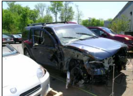
Figure 5. Front and right damage from the first utility pole impact.
