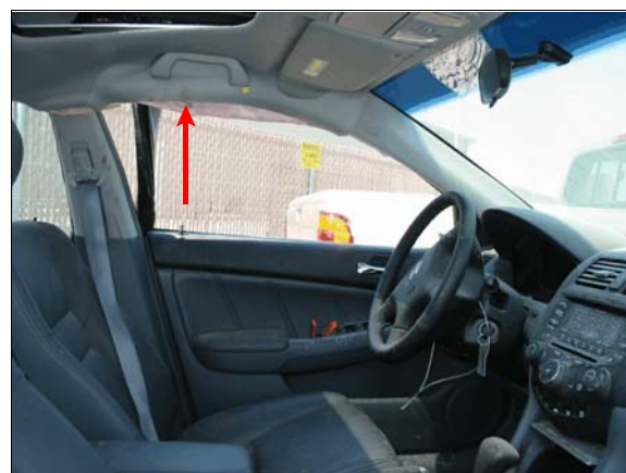
Figure 10: Overview of driver’s door, steering wheel , left instrument panel and left portion of windshield, arrow shows reddish brown scuff mark on roof side rail.
