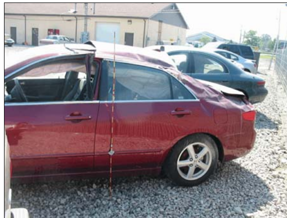
Figure 3: Damage to case vehicle's left roof side rail and left "C"-pillar from ground impact, each increment on rods is 5 cm (2 in)
