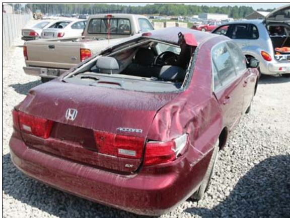
Figure 6: Overview of back and right side showing rollover damage to right quarter panel and left "C"-pillar, roof and left roof side rail
