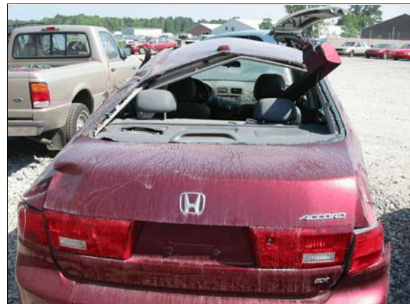
Figure 7: Back view of crush to left "C"-pillar and roof side rail
