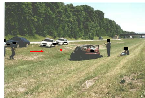
Figure 4: View southeast to case vehicle's rest position, arrows show case vehicle's tire furrows in grass
