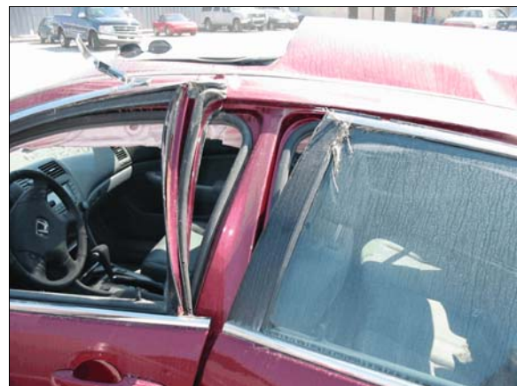
Figure 9: Rollover damage to left front and left rear doors
