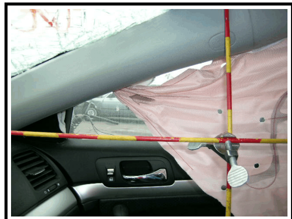
Figure 22. Gap distance after tether pulled out of the A pillar cover
