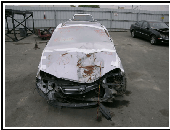
Figure 1. Front end damage - 2005 Acura TSX
