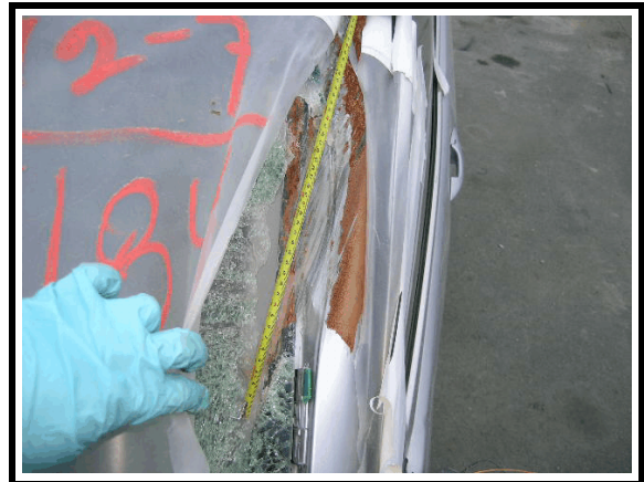
Figure 14. Closer view - Left A pillar damage
