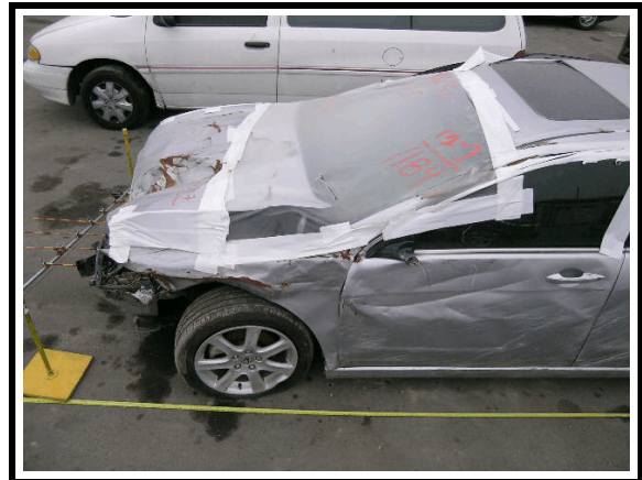
Figure 13. Left front rollover damage and left A pillar damage
