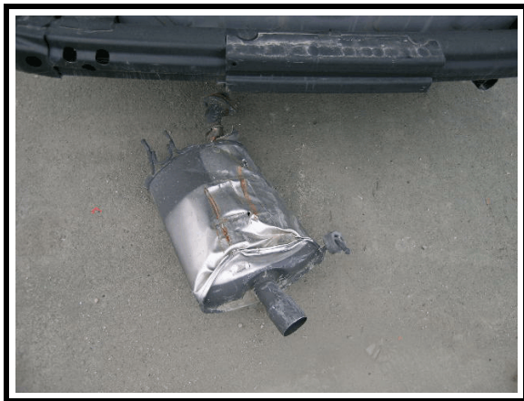
Figure 12. Damaged left muffler
