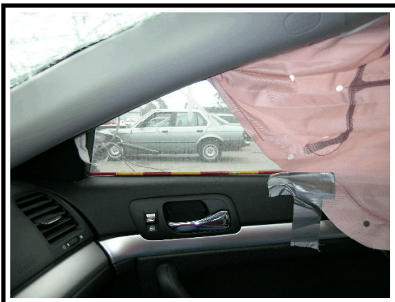
Figure 21. Gap distance at Right A pillar as found at the inspection
