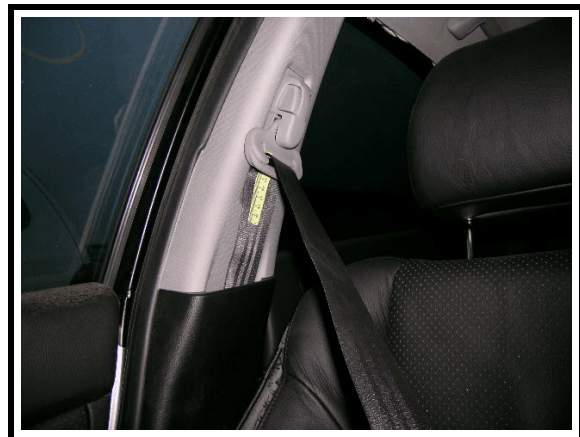
Figure 25. Evidence of loading to the right front passenger's seat belt
