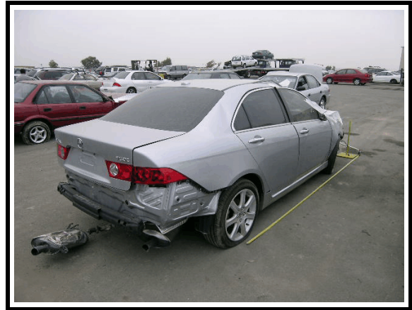
Figure 11. Back/right and muffler damage from undercarriage impact
