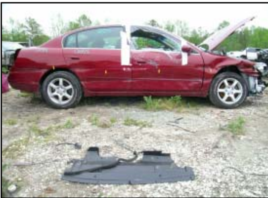
Figure 2. Right sideswipe damage from the initial guardrail impact.
