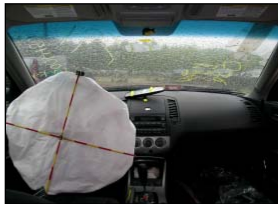
Figure 7. Deployed driver's frontal air bag.
