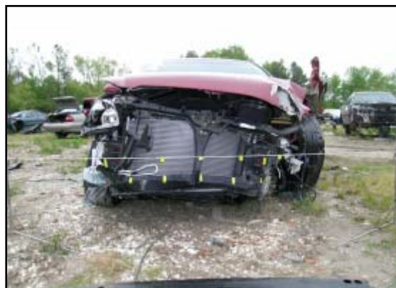
Figure 4. Frontal damage from the second guardrail impact.
