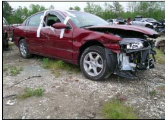
Figure 3. Front right damage from the initial guardrail impact.
