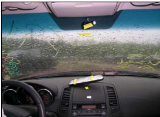
Figure 5. Rear view mirror contact point.
