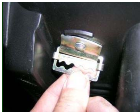
Figure 10. Close-up view of the buckle and saw-tooth locking bar.
