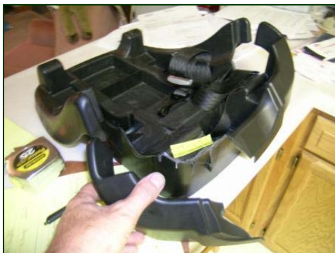
Figure 7. Fractured base at LATCH belt path.
