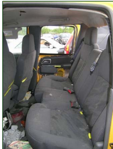
Figure 13. Trajectory of the infant and contact damage to the right rear door panel.
