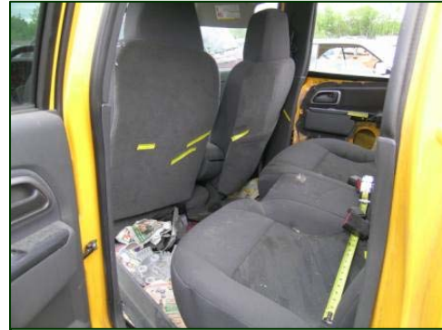
Figure 6. Lateral view of the rear seat area damage and intrusion.
