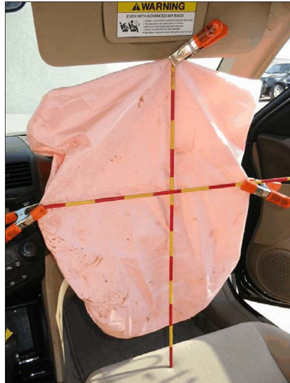
Figure 13: Case vehicle's front right passenger air bag, air bag has numerous stains on it, they appeared to be coffee stains
