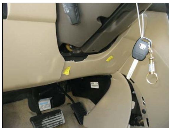
Figure 15: Case vehicle driver's knees impacted and broke the drivers knee bolster
