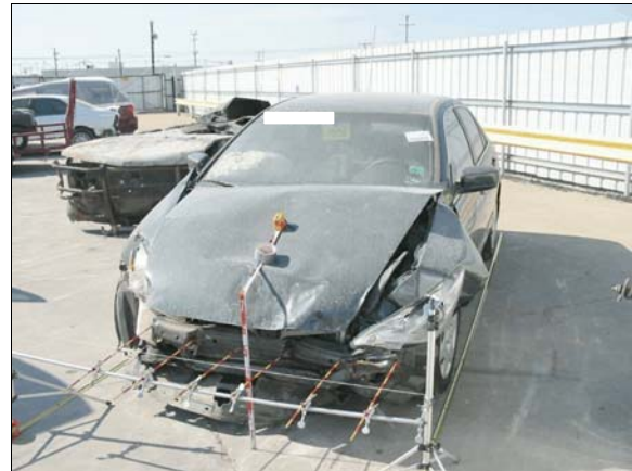
Figure 4: Front left overview of damage to case vehicle, each number on tape measure is tenths of meter, each stripe on rods is 5 cm (2 in)
