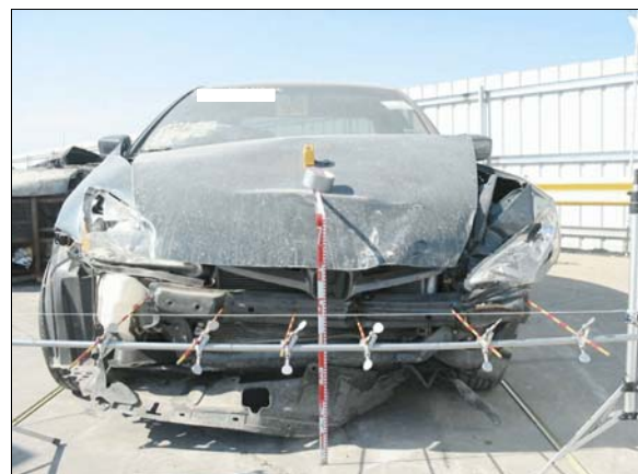
Figure 5: Damage to front of case vehicle from impact with the other vehicle
