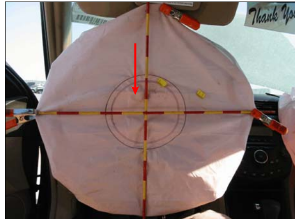
Figure 11: Case vehicle driver's air bag, arrow shows location of possible lip imprint, yellow tape shows locations of stain, they did not appear to be related to occupant contact
