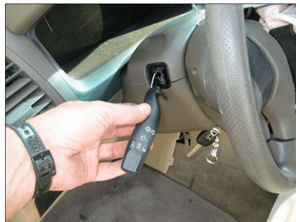
Figure 14: Case vehicle driver's left hand impacted and broke the turn signal lever off the steering column
