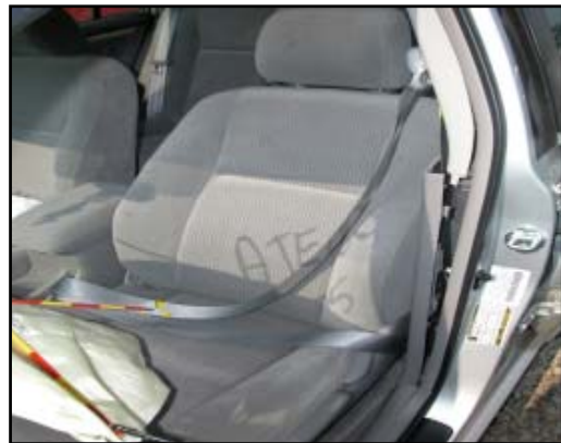
Figure 10. Driver's safety belt restricted in the used position.
