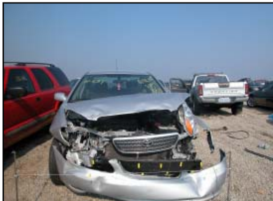
Figure 6. Resultant damage to the frontal plane of the Toyota.
