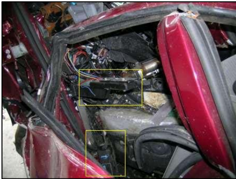
Figure 3. Adaptive throttle and brake hand control, separated from mount.
