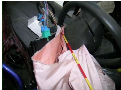
Figure 12. Tear of the driver's air bag.
