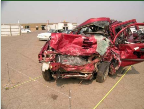
Figure 10. Frontal view of the damage to the Ford Windstar.
