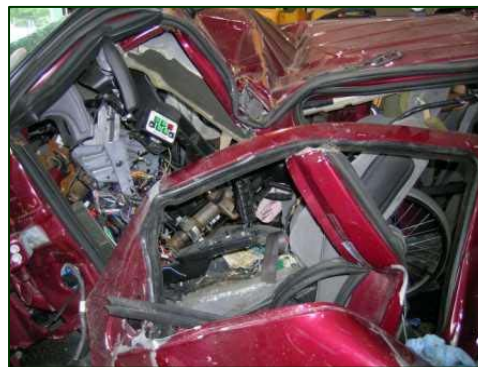
Figure 14. Intrusion of the driver’s compartment.
