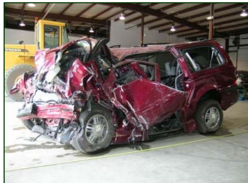
Figure 8. Compression of the frontal structure and of the driver's compartment.
