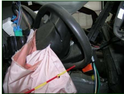
Figure 9. Deformed upper steering wheel rim.
