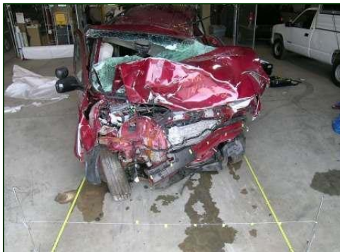
Figure 7. Overhead view depicting the extend of frontal crush.
