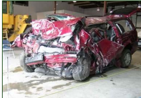
Figure 1. Severe frontal damage to the 2005 Chevrolet Venture adaptive control minivan.
