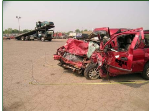
Figure 11. Lateral view of the Windstar's frontal crush profile.
