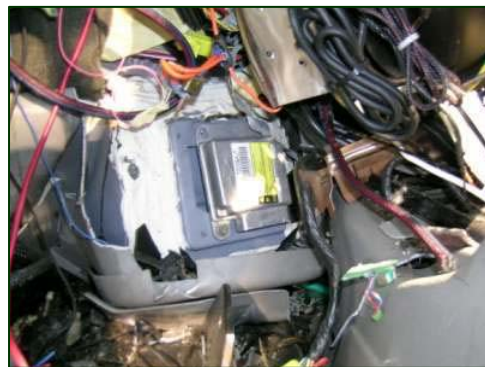
Figure 13. Repositioned and rotated SDM by intrusion.
