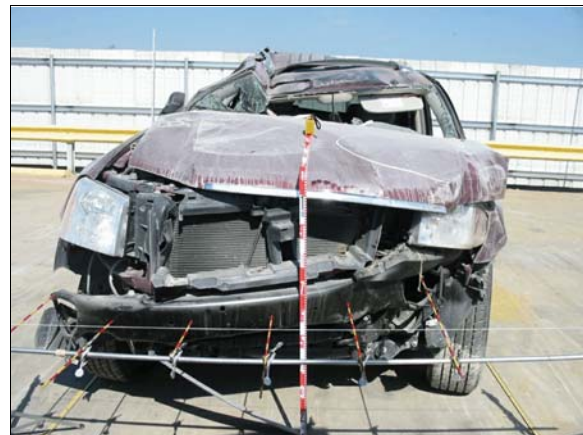
Figure 2: Damage to front of case vehicle from impact with concrete median barrier and to the roof from the rollover, numbers on tape measure on hood are tenths of meter
