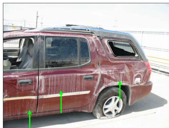
Figure 7: Rollover damage to left side of case vehicle, vertical streaks indicated by arrows are not rollover damage, they are streaks in dust from rain runoff
