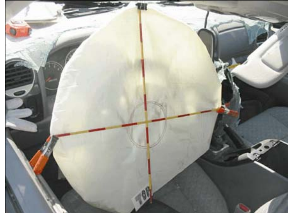
Figure 13: Case vehicle's driver air bag, steering wheel is rotated 180 degrees, top of air bag is at bottom of photo
