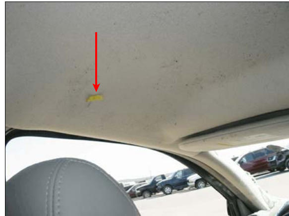
Figure 10: Arrow shows area of hair deposit on roof above driver’s seat
