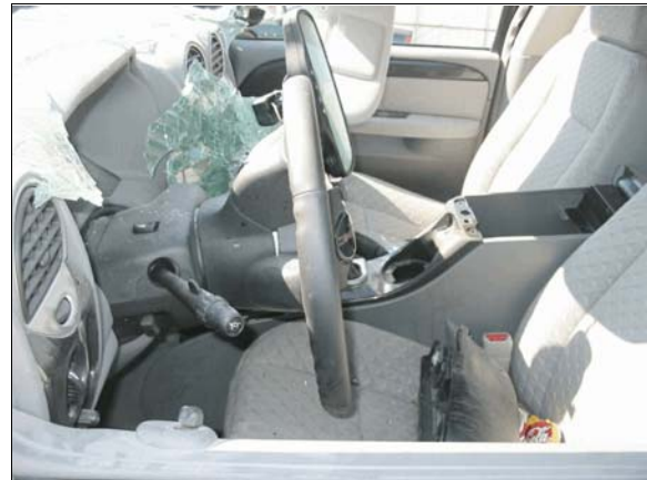
Figure 11: Left side view of case vehicle’s steering wheel and steering column showing lack of deformation
