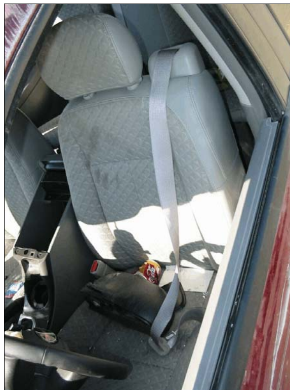
Figure 15: Overview of driver's seat and safety belt, the safety belt was partially out of the retractor and the retractor was jammed
