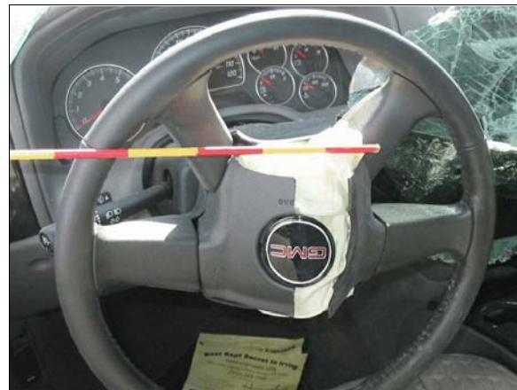
Figure 12: Case vehicle driver’s air bag module cover flaps, each stripe on rod is 5 cm (2 in)
