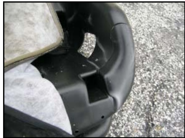
Figure 15: View of the fractured shell.
