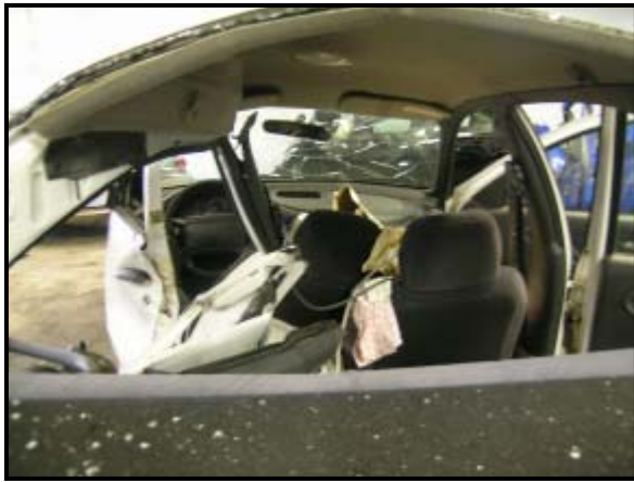
Figure 10: View through the backlight of the extent of the intrusion.
