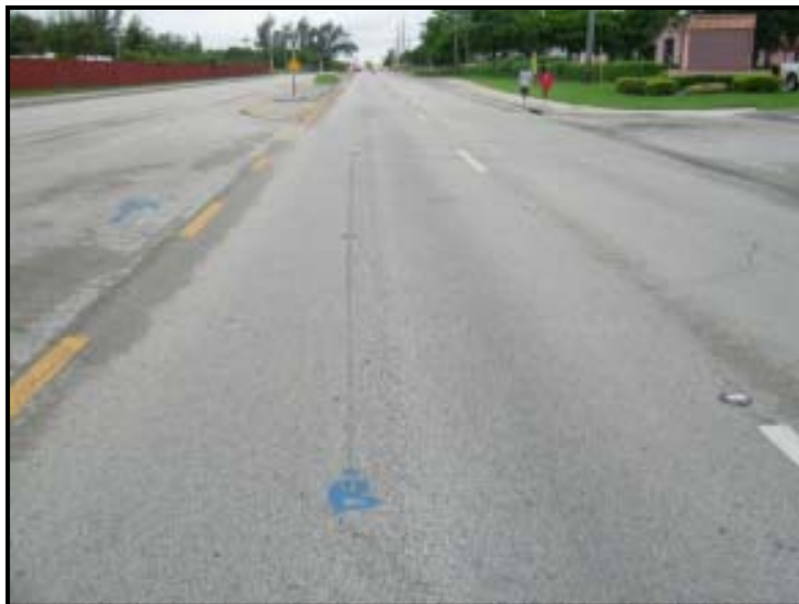
Figure 7: Trajectory view of the motorcycle and the west skid leading to the point of impact.
