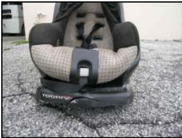
Figure 14: Front view of the fractured CSS.
