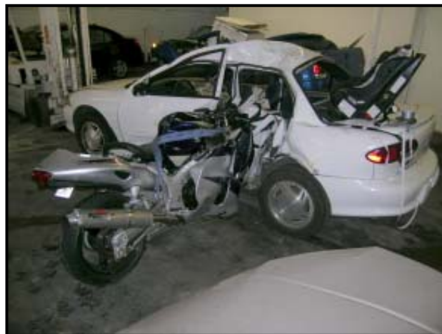
Figure 8: View of the impact configuration.
