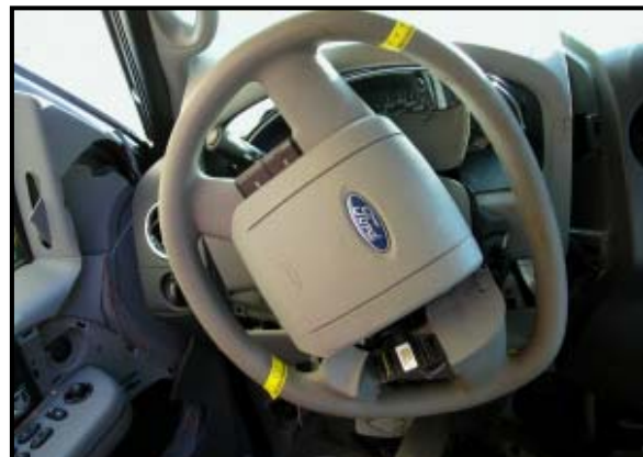
Figure 11: Deformed steering wheel rim and undeployed driver air bag module.
