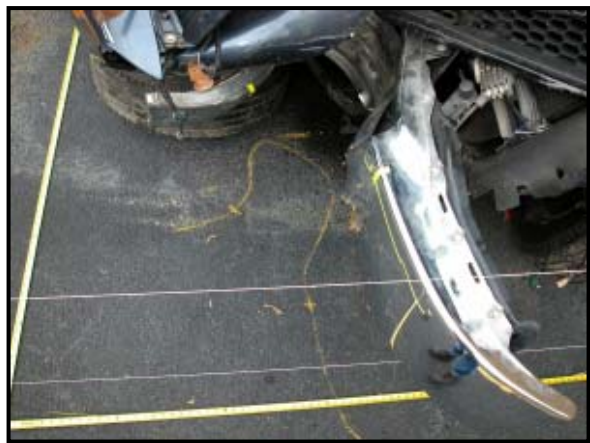
Figure 8: Overhead view of the bumper deformation.
