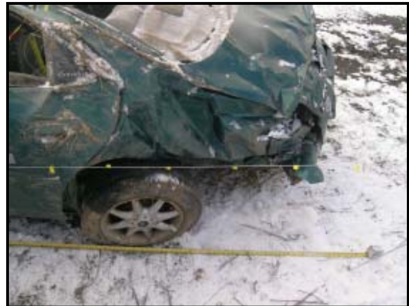
Figure 7: Left rear quarterpanel deformation.
