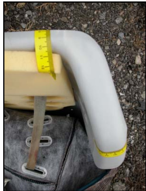
Figure 16: Minor stress marks on left wing of the CSS shell.
