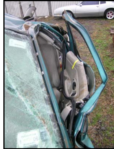
Figure 9: View of the driver's ejection path.
