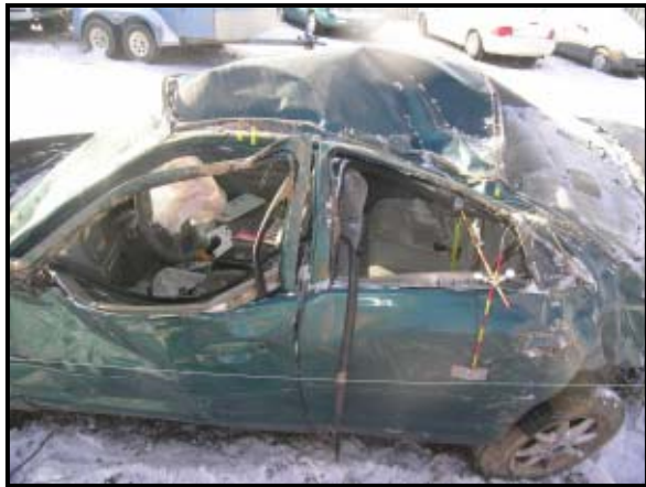
Figure 6: Left view of the roof deformation.
