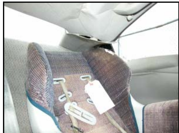
Figure 11: Top aspect of the CSS and intruded trim.
