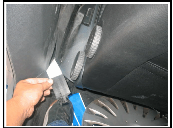
Figure 15. Driver's seat belt - cut by fire/rescue personnel
