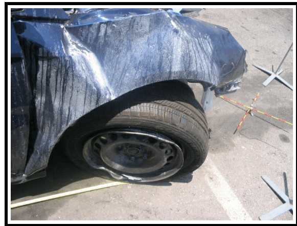
Figure 8. Right front tire & rim damage
