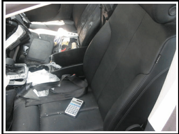
Figure 12. Driver's seat belt, cut by fire/rescue personnel
