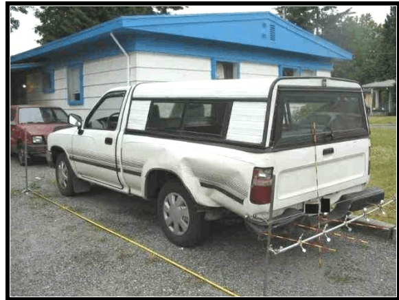
Figure 5. Rear damage, 1993 Toyota pickup
