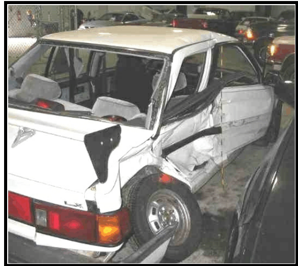
Figure 1. Right side damage, Honda Civic
