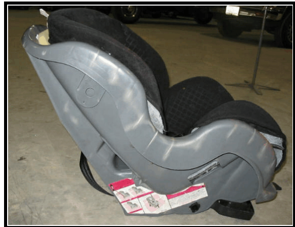
Figure 13. Right side loading damage
