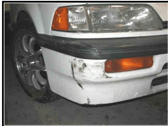
Figure 7. Honda Civic, front right bumper corner damage
