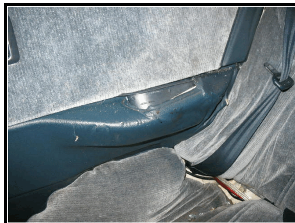
Figure 8. Intrusion at second row right door
