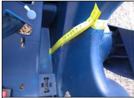
Figure 13. Fracture at the carry handle.
