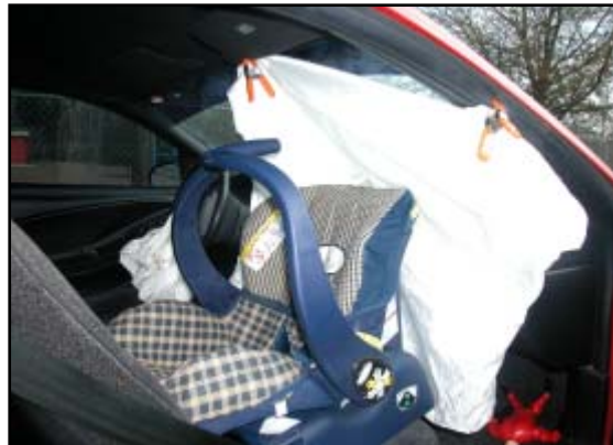
Figure 11. Expansion of the air bag membrane against the RFCSS.
