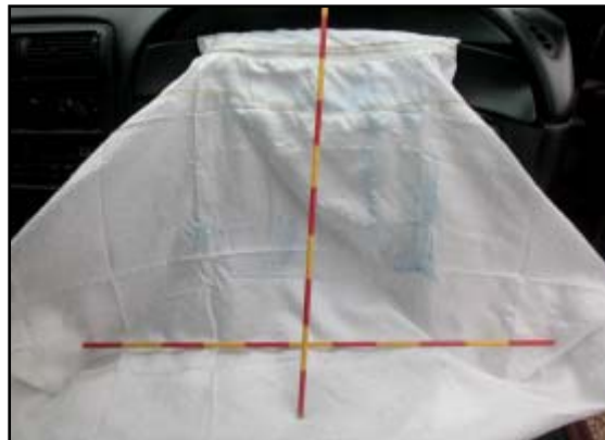
Figure 9. Blue plastic transfer on the top panel of the air bag membrane.
