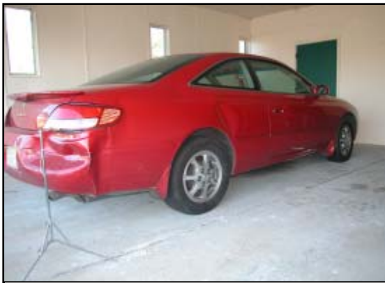
Figure 5. Resultant damage to the rear of the Toyota.
