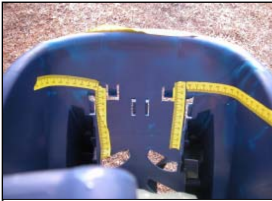
Figure 12. Fractures at the top of the RFCSS.
