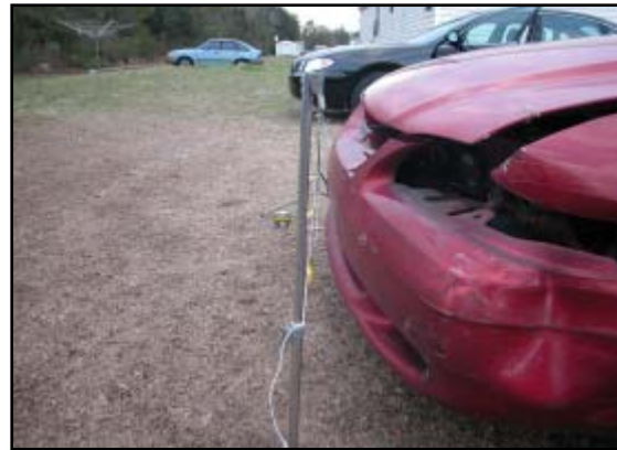
Figure 4. Lateral view of the crush profile
