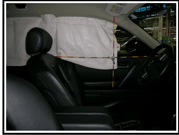
Figure 12. Left side curtain air bag
