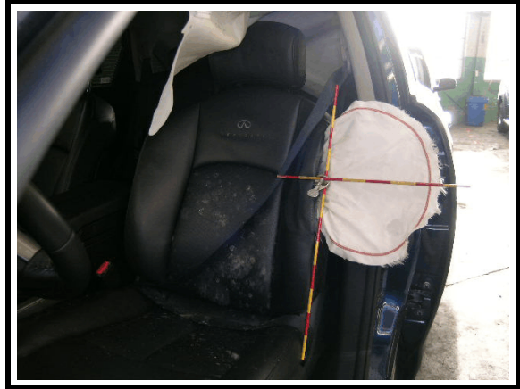
Figure 11. Driver's seat back mounted side air bag
