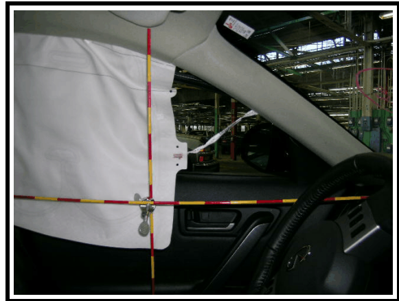
Figure 13. Left side curtain gap distance at the left A pillar.
