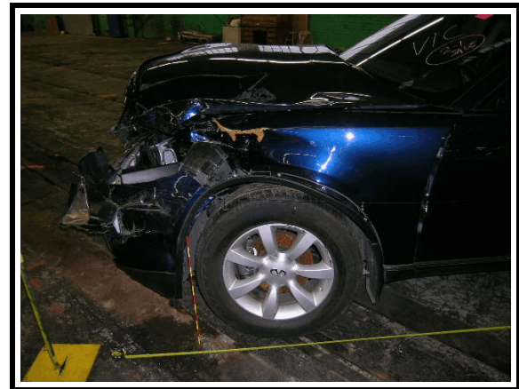
Figure 9. Direct damage - 2005 Infiniti FX35
