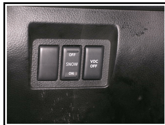
Figure 7. VDC and Snow Mode switches
