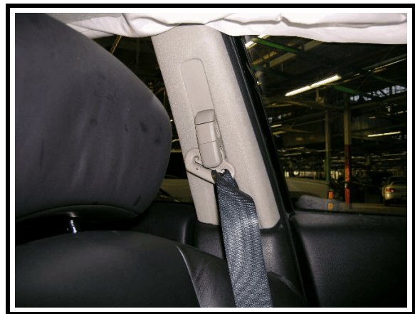
Figure 10. Driver's seat belt - cinched in D ring. B-pillar pretensioner actuated.
