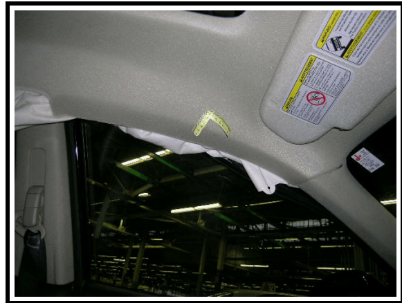
Figure 14. Occupant contact/hair transfer to left roof side rail
