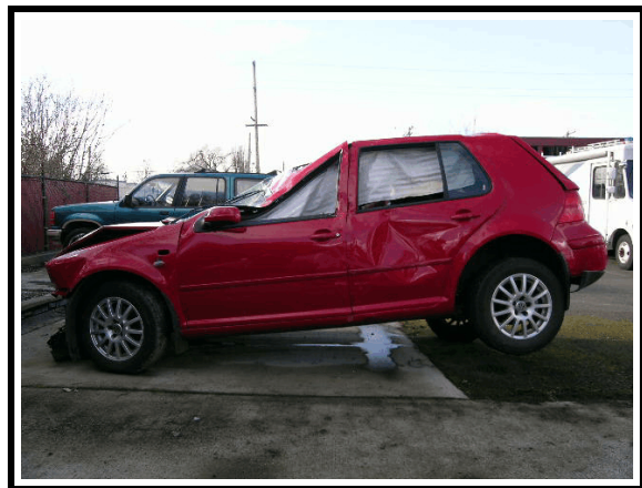
Figure 2. Left side damage - 2003 Volkswagen Golf
