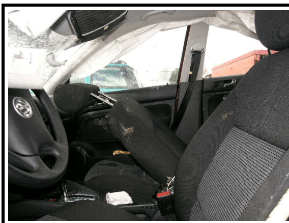
Figure 29. Damaged front right seat back - locked in this position
