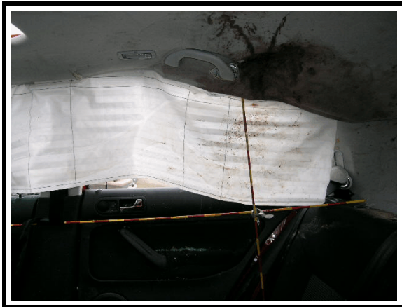
Figure 24. Back section of the right side curtain
