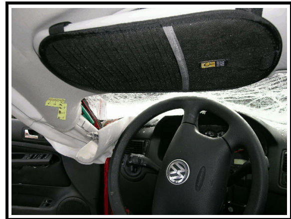
Figure 26. Possible occupant contact to top of left A pillar
