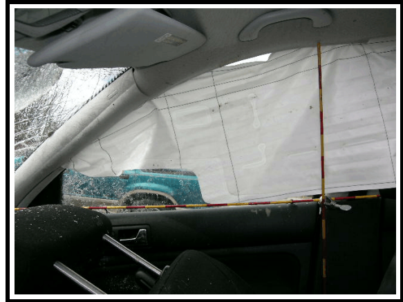
Figure 23. Right side curtain gap distance at the right A pillar
