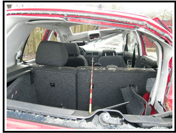
Figure 16. Passenger compartment damage/intrusion
