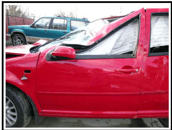
Figure 13. Left A, B pillar and LF door damage
