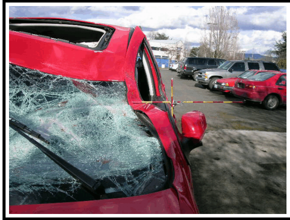
Figure 14. A pillar damage from tree impact - occurred during the rollover event
