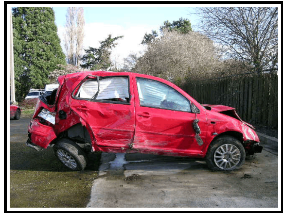
Figure 1. Right side damage - 2003 Volkswagen Golf
