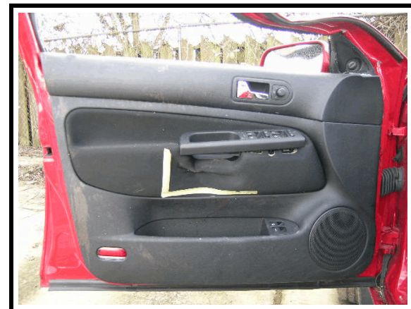
Figure 27. Deformation to LF door armrest
