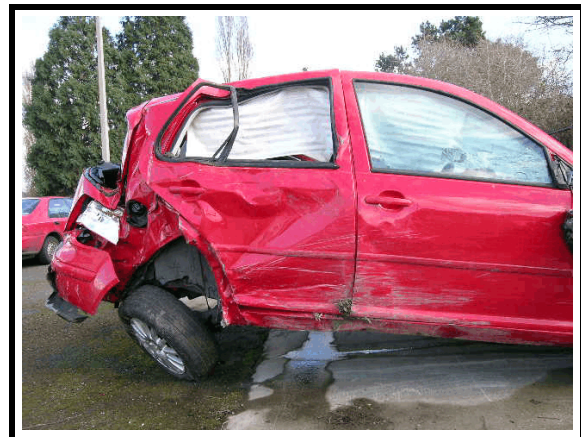
Figure 11. Right rear damage
