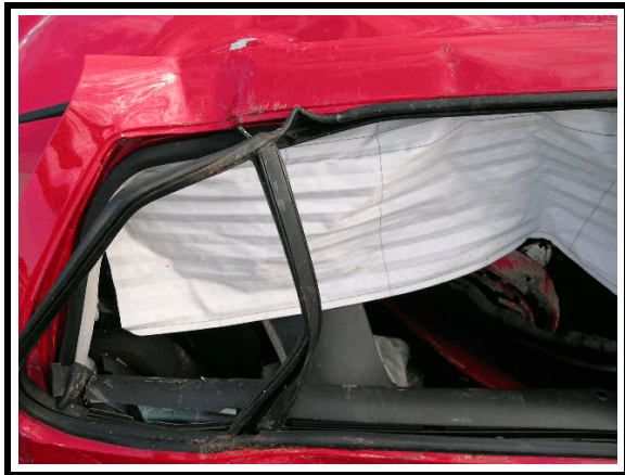
Figure 36. Deformed right rear window frame
