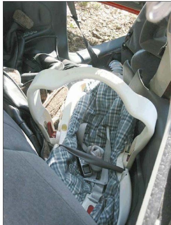
Figure 16: Top view of back right passenger's infant seat showing extent of intrusion of right "B" pillar and side panel rear of "B"-pillar.
