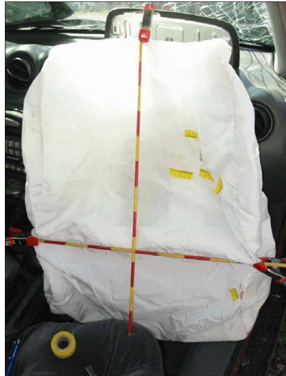
Figure 12: Overview of case vehicle's front right passenger's air bag
