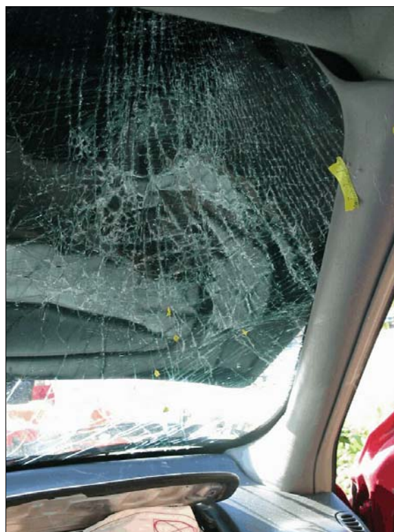
Figure 17: Overview of driver's head impact to windshield and right "A"-pillar, yellow tape shows hair adhering to windshield and contact mark to right "A"-pillar
