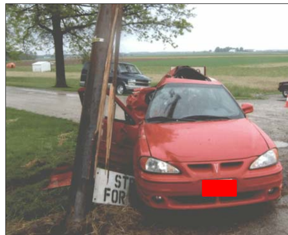
Figure 5: Police on-scene photo showing case vehicle's final rest position and post-impact condition of utility pole
