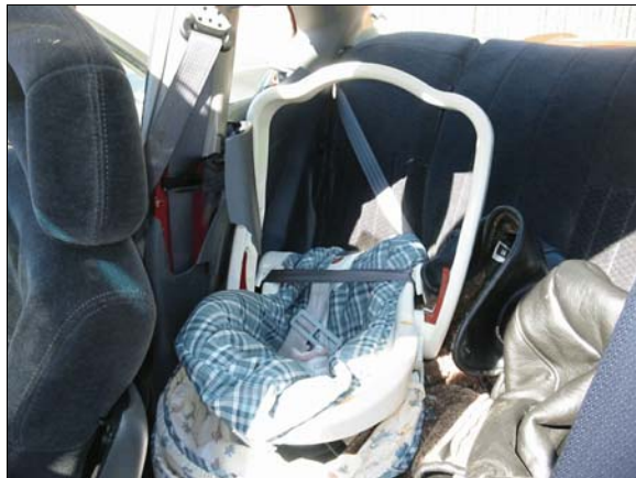
Figure 15: Overview of back right passenger's rear-facing infant seat as found in the case vehicle
