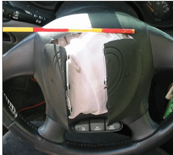
Figure 9: Overview of driver's air bag module cover flaps, each increment on rod is 5 cm (2 in)
