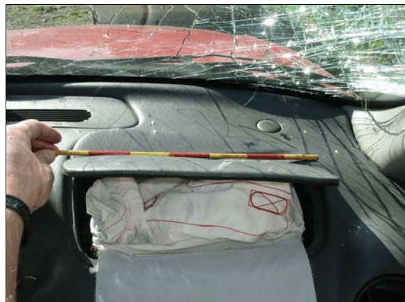
Figure 11: Front right passenger air bag module cover flap
