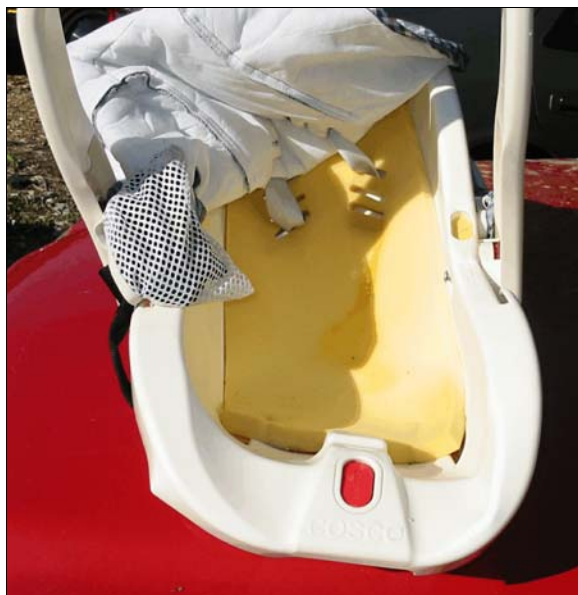
Figure 18: Front view of infant seat showing bending of the seat due to loading by the case vehicle's intruding right "B"-pillar and side surface rear of the "B"-pillar
