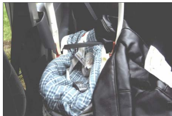
Figure 17: Police on-scene photo showing post-crash condition of back right passenger's infant seat
