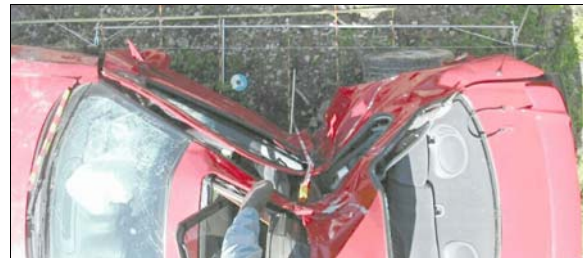
Figure 7: Top view of crush to right side of case vehicle due to utility pole impact
