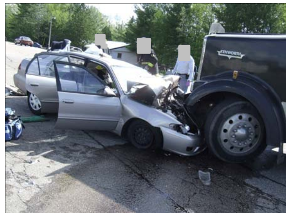
Figure 6: View southwest showing case vehicle's underride of front of Kenworth
