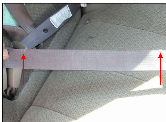
Figure 21: Arrows show load marks on back right passenger safety belt, photo view from top left
