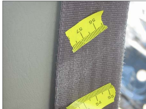
Figure 18: Load mark on driver's shoulder belt
