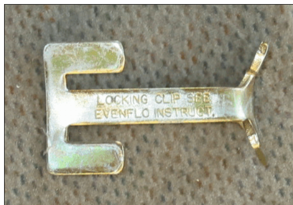
Figure 20: Deformed safety belt locking clip for back right child safety seat
