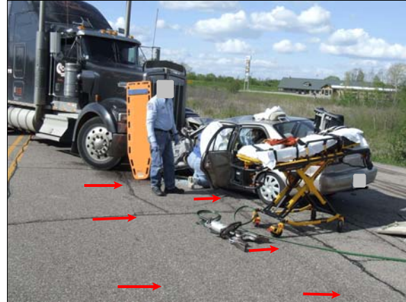
Figure 3: Police on-scene photo showing rest positions of case vehicle and Kenworth, arrows show case vehicle's pre-impact skid marks
