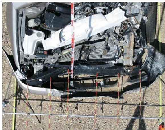
Figure 8: Top view of crush to case vehicle's front bumper
