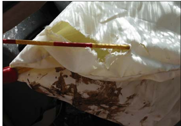
Figure 12: Close view of tear in driver's air bag
