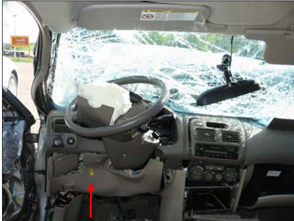
Figure 10: Overview of steering wheel, instrument panel and windshield, arrow shows deformation of driver's knee bolster
