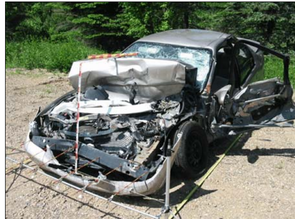
Figure 5: Damage to front of case vehicle from impact with the Kenworth, each increment on rods is 5 cm (2 in), vertical scale is graduated in tenths of meter
