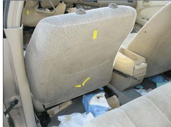
Figure 11: Yellow tape shows probable occupant contact marks from back left passenger on the back of the driver's seat
