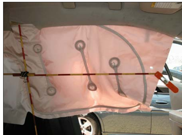
Figure 10: Forward section of left side curtain air bag, each increment on rods is 5 cm (2in)
