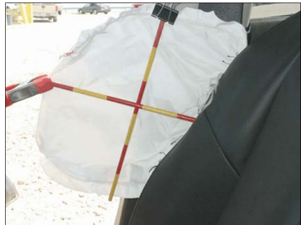
Figure 12: Front right seat back-mounted side impact air bag
