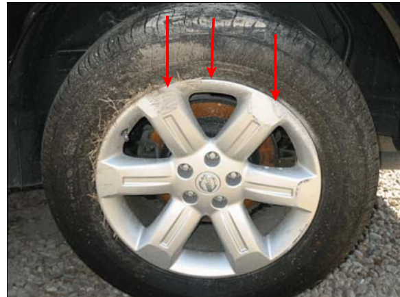
Figure 4: Arrows show rim abrasions to left rear wheel from gouging roadway surface, gras was also jammed in bead when case vehicle rotated clockwise off tree stump impact
