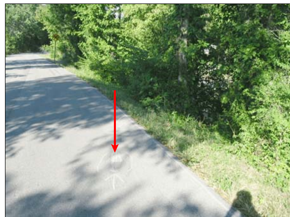
Figure 5: Left rear wheel gouge in roadway (arrow) and embankment case vehicle rolled down
