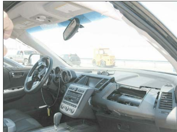
Figure 9: Case vehicle's instrument panel, windshield and steering wheel, driver and front right air bag modules had been removed, probably for salvage
