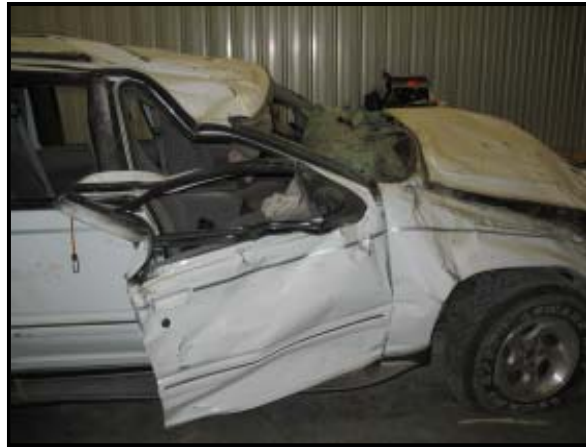
Figure 6: Maximum crush in the right A-pillar area.
