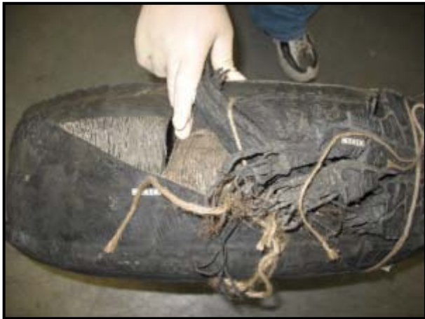
Figure 10: Casing damage at 330 degrees
