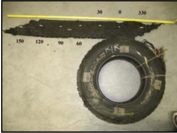
Figure 7: Overall view of tire and detread. Non DOT side shown.
