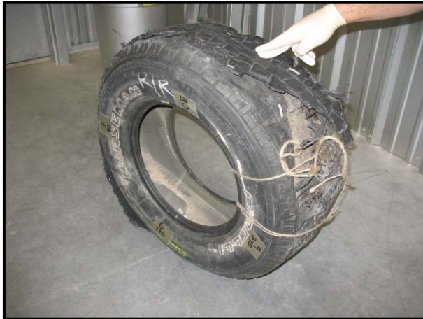
Figure 9: Detread section and tire.
