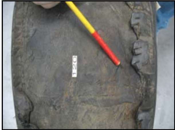
Figure 14: Close-up of tire at the construction seam. Note the nail location.
