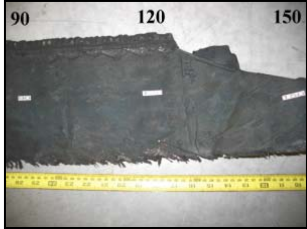
Figure 12: Detread section (interior side).
