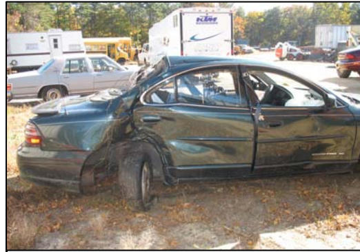
Figure 7 - Damaged right side of 2000 Pontiac Grand Prix.
