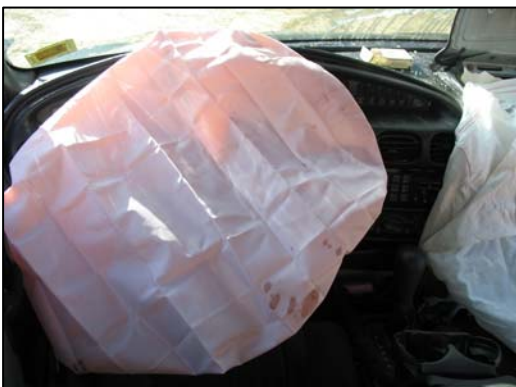
Figure 8 - Deployed driver's air bag.
