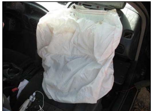
Figure 9 - Deployed front right air bag.
