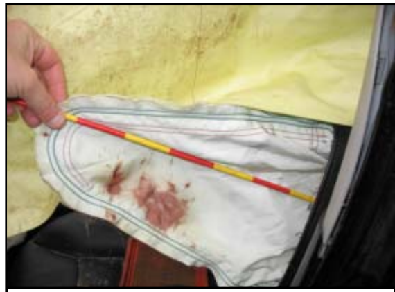
Figure 9. Deployed driver's seatback mounted side impact air bag.
