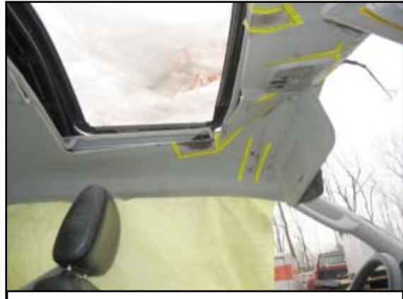
Figure 7. Overall view of the front roof and windshield header contact points.
