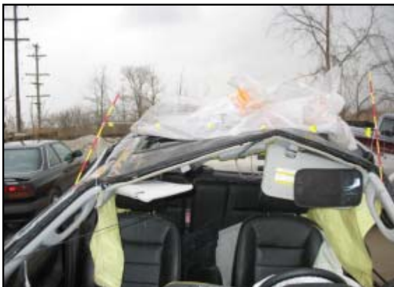
Figure 5. Vertical crush profile at the windshield header.
