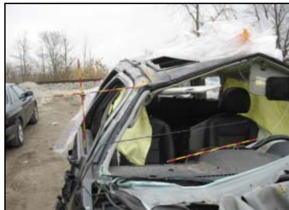
Figure 6. Location of maximum vertical and lateral crush at the A-pillar area.
