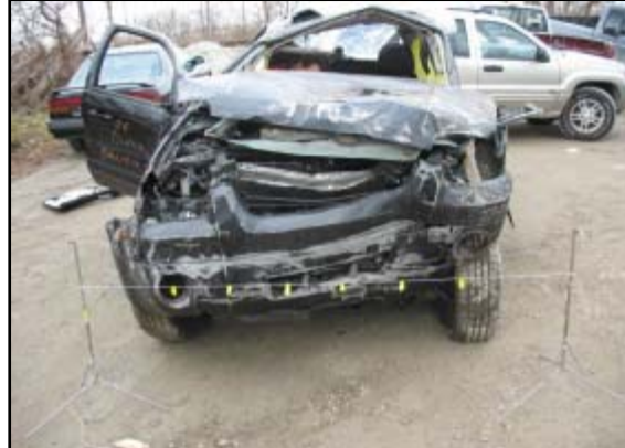
Figure 4. Resultant frontal damage.
